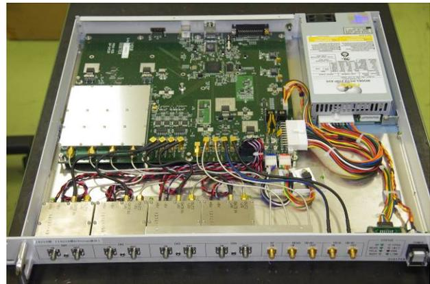
Figure 8: Photo of the 1421B gated turn-by-turn monitor.
