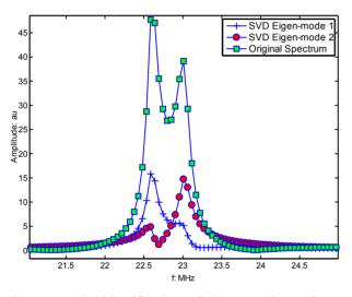
Figure 7: The identification of SVD modes and two polarizations of a dipole signal.
