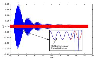
Figure 2: Dipole signal from HOM coupler 2 of 1<sup>st</sup> cavity at module 5. The calibration signal is highlighted with red colour and has a pure sinusoidal waveform.
