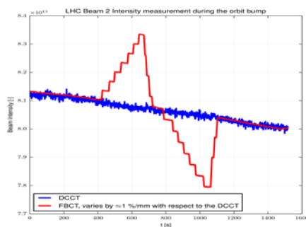
Figure 1: Beam position dependency in present LHC FBCTs with an orbit bump of \pm 4 mm.
