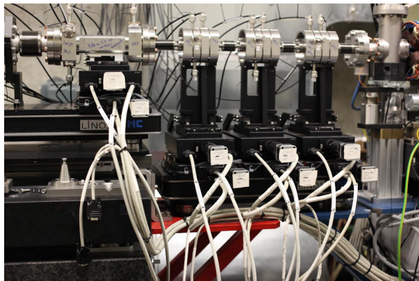
Figure 1: CBPM test-stand at FLASH1 with three undulator CBPMs (right) and one 40.5 mm beam pipe diameter CBPM (left). The beam passes the pickups from right to left. Each CBPM can be moved in both transverse directions with remote movers.
