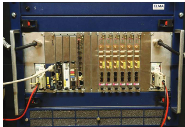
Figure 1: MTCA.4 crate equipped with AMC cards.
