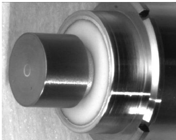
Figure 3: Photograph showing one unit with the 6x4mm button, its central pin welding and its support to the ceramic, and the UHV side of the housing.
