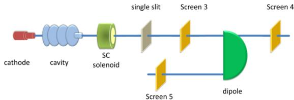
Figure 2: Diagnostics beamline for ELBE SRF gun II.
