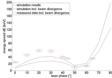
Figure 4: Measured and simulated energy spread with different laser phase.
