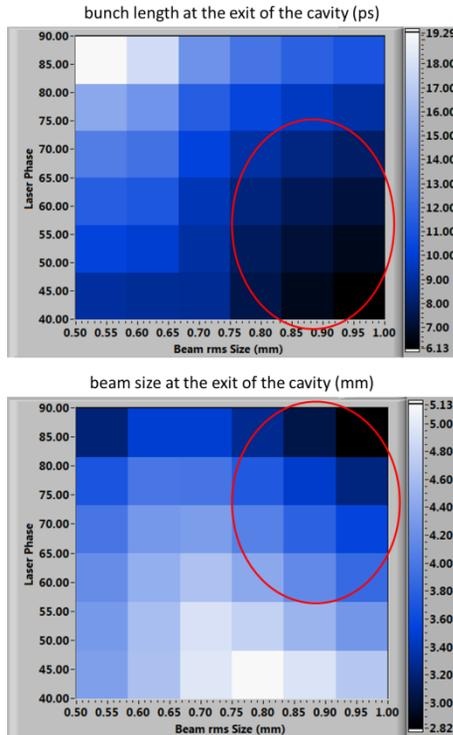
Figure 6: Simulation results: Expansion of the 3D bunch size at the exit of the SRF gun versus initial beam size. Different laser phases are scanned. Red areas are proper parameters.
