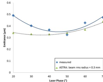
Figure 5: Transverse emittance versus laser phase.
