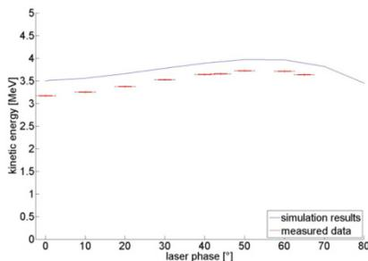
Figure 3: Measured and simulated kinetic energy of the beam versus laser phase.
