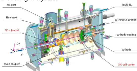
Figure 1: construction of the ELBE SRF Gun II.
