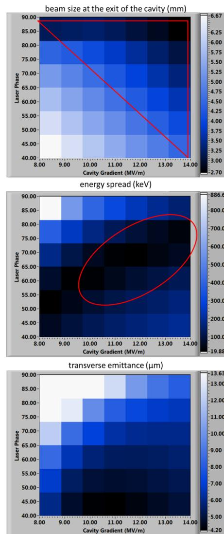
Figure 7: Simulation results: RF gradient and laser phase scanning for the beam with bunch charge of 1 nC. Results are given for the exit of the SRF cavity.
