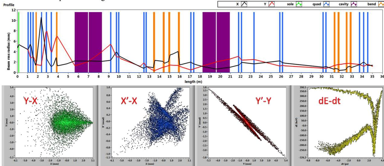
Figure 8: Beam transport and phase spaces of 1nC, 10MV/m. The massive X phase space is due to the CSR effect and the nonlinear longitudinal phase space is the result of LSC effect and the bunching of the chicanes.
