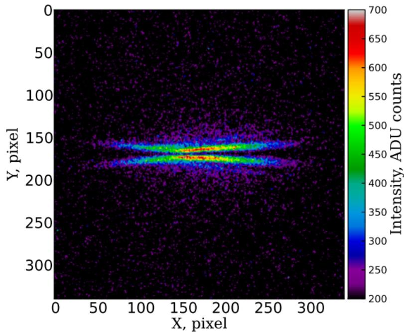
Image of the OTR spot taken with linear polarizer and  $550 \pm 20$  nm optical filter
