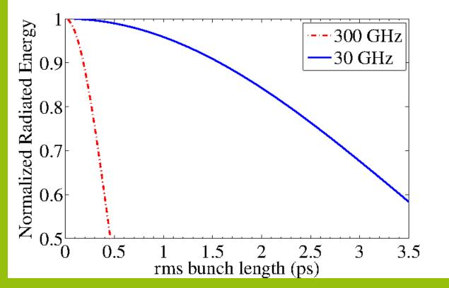
Energy radiated by a rectangular electron bunch at 30 and 300 GHz
