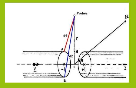
GAP → Faced coaxial waveguides Charge passes through the gap → currents induced on the pipe walls → Source for electromagnetic field Both from Step-out and Step-in
