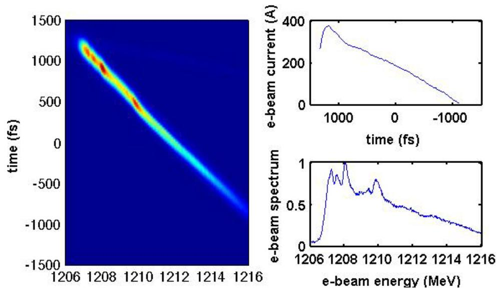
In specific configurations of the linac the electron beam measured at the end of the accelerator shows **strong linear correlation**.
