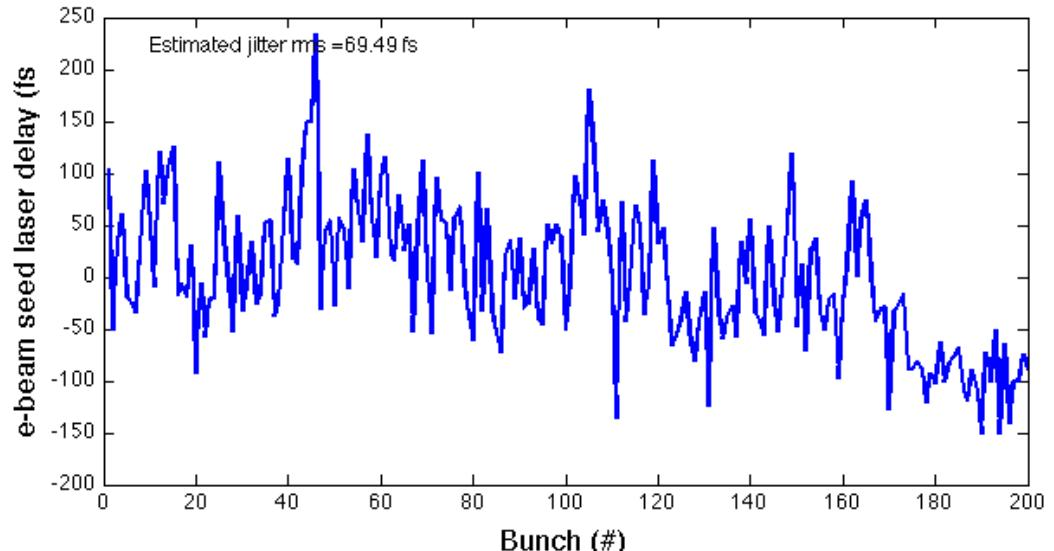
By measuring the evolution of the “hole” we can measure the **changes** in the relative timing between the electron and seed laser for each shot.
