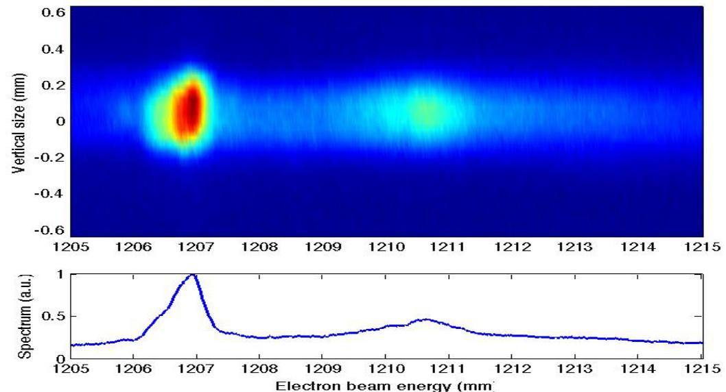
*Measured electron beam spectrum at MBD for the beam not seeded.*
