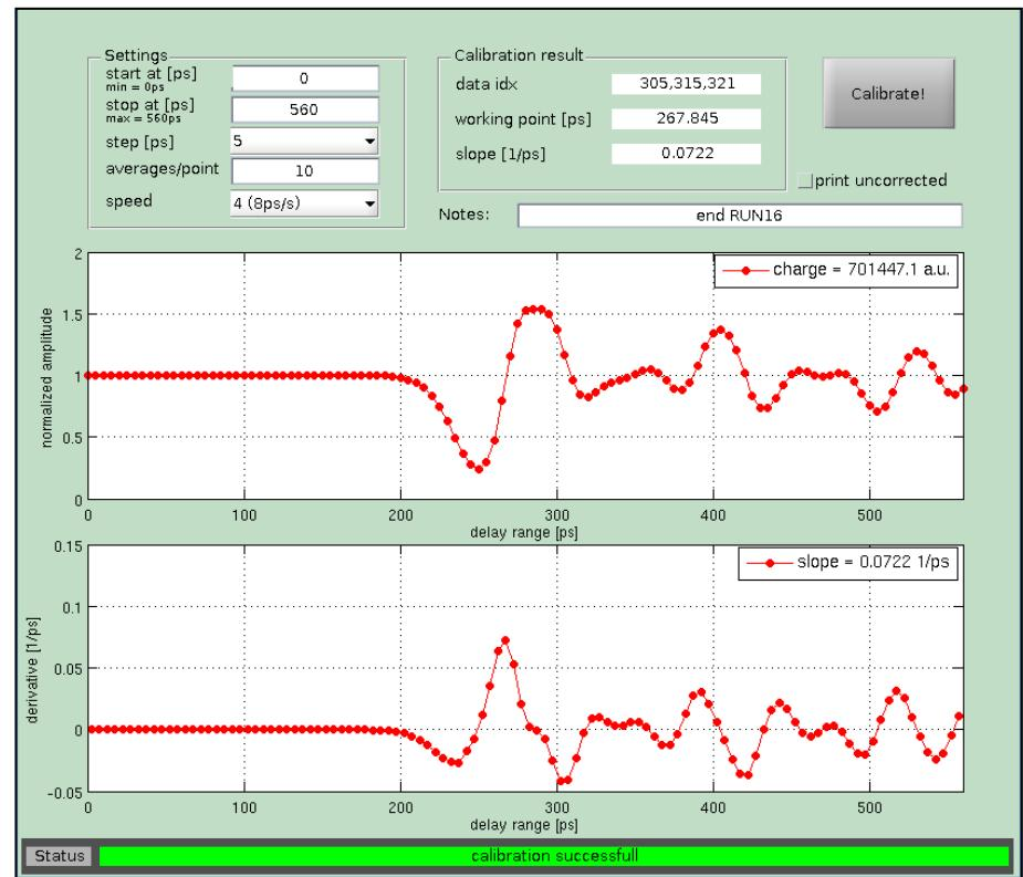
BAM calibration via optical delay line scan of the reference laser pulse over the BAM pick-up signal.
