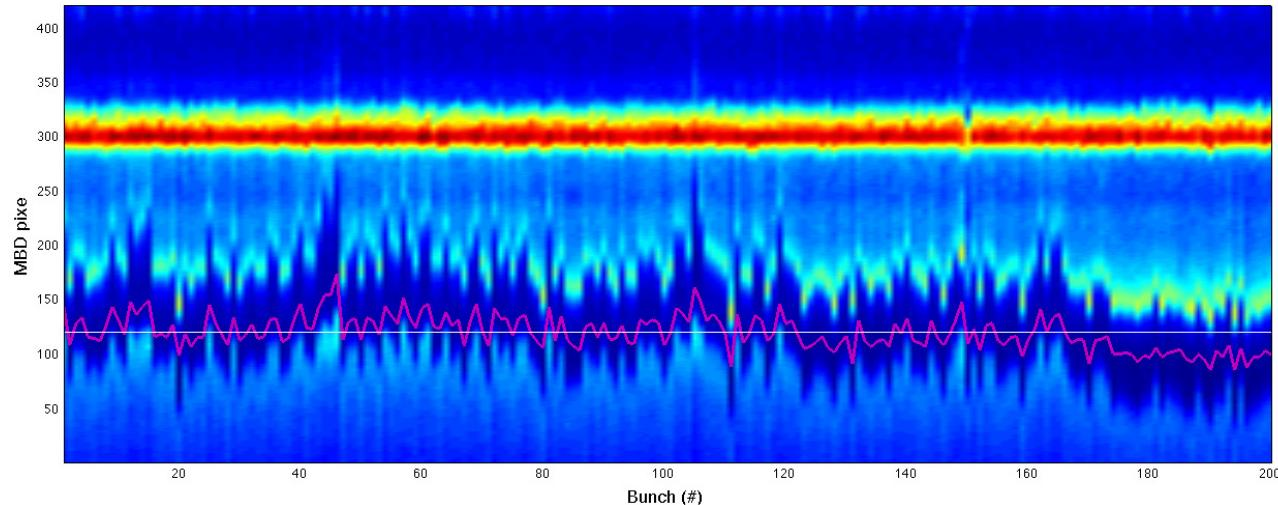
*Sequence of 200 seeded electron beam spectra measured in MBD. While the peak is fixed in energy, the position of the seed induced “hole” is moving.*
