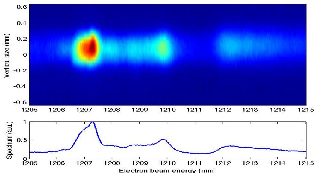
*Measured electron beam spectrum at MBD for the beam seeded.*
