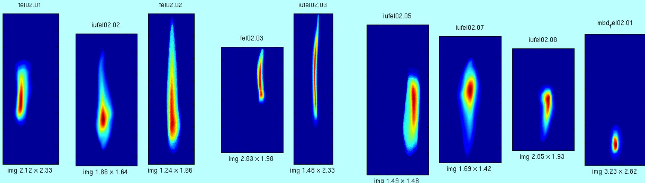
Envelope reconstruction along the undulator chain with **deflected beam** (e.g.: transverse wakefield compensation check).
