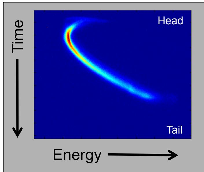
Coupled RF deflector (vertical) and dipole spectrometer (horizontal)
