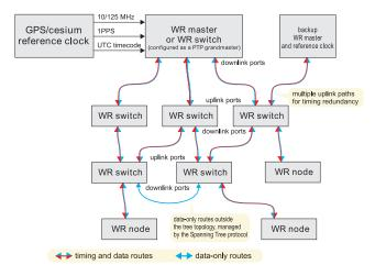
Links are 1Gb/s single fibre (TX and RX use different wavelengths).
