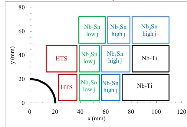
**Magnet design: 40 mm bore (depends on injection energy: > 1 Tev)**
