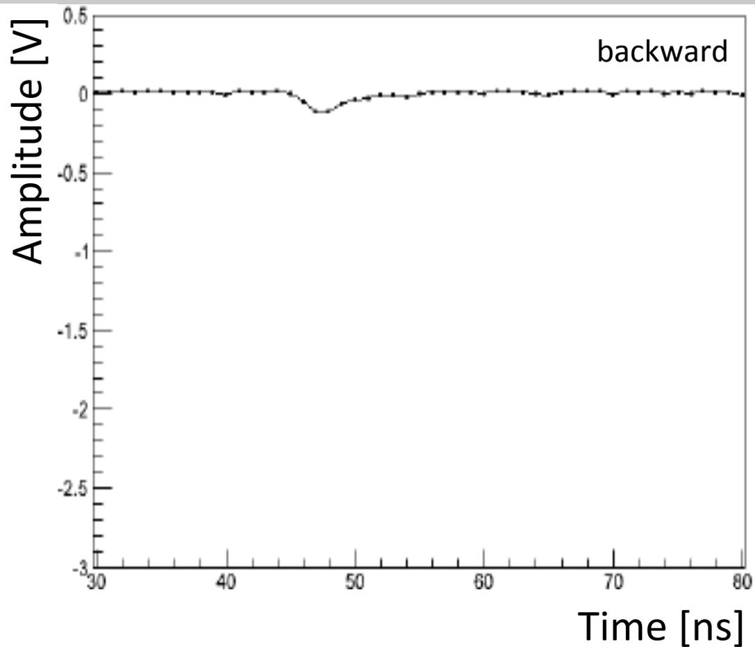
Example waveform from muon arriving under 150deg.
