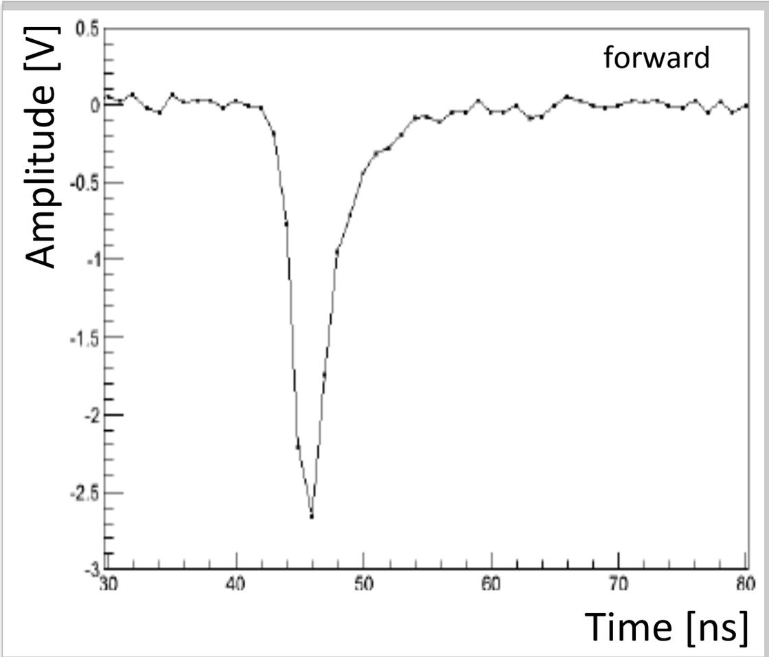
Example waveform from muon arriving under 30deg.
