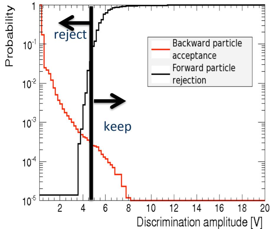
Accumulative (0deg) and Inverse accumulative (180deg) amplitude distributions
