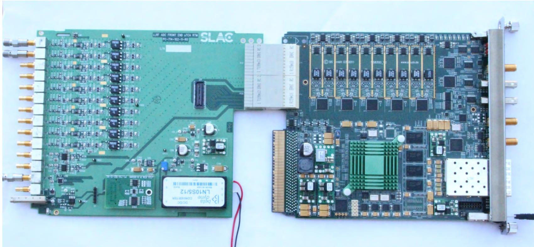
Using the LLRF RTM board with a modification for MPS interface we can interface with the Struck 119MSa/s ADC. Using the general DIO bit on Zone 3 connector we can design an MPS TTL logic interface.
