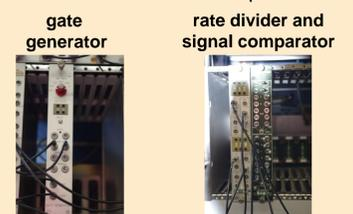
Fig. 7. NIM modules used for multi-triggering
