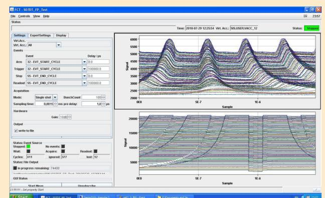
Fig. 8. Beam profiles and RF reference timing measured during acceleration. The time between two consecutive events is 3000 revolutions. The vertical axis represents the time in arbitrary units along the machine cycle.
