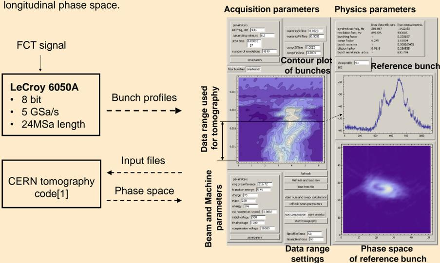
Fig. 1. Tomography diagnostics scheme in the SIS 18.
