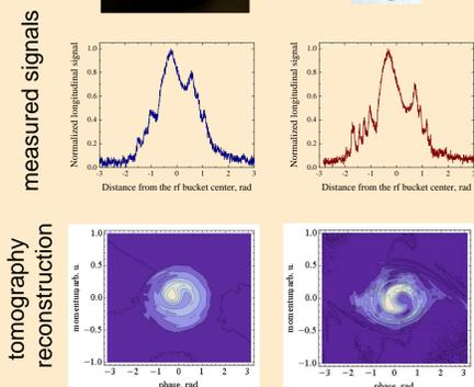
Fig. 5. Comparison of the data from the wide band FCT and position pick-up
