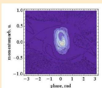
Fig. 4. Reconstructed phase space of the compressed bunch
