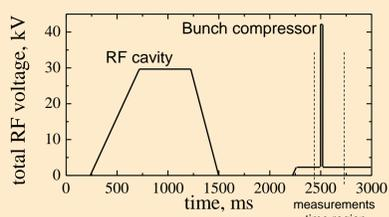
Fig. 2. Schematic RF cycle in SIS18 with bunch compression
