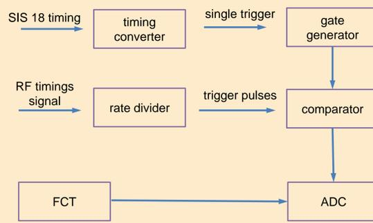
Fig.6. Schematic hardware setup for multi-events measurements
