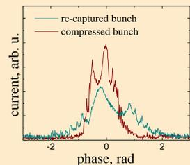
Fig. 3. Bunch profile before and after compression
