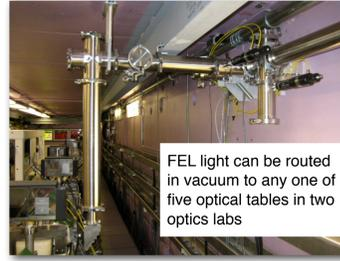
FEL light can be routed in vacuum to any one of five optical tables in two optics labs
