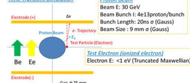
Beam induced electric field at the time of bunch peak: E<sub>max</sub>: 1.6e5V/m
