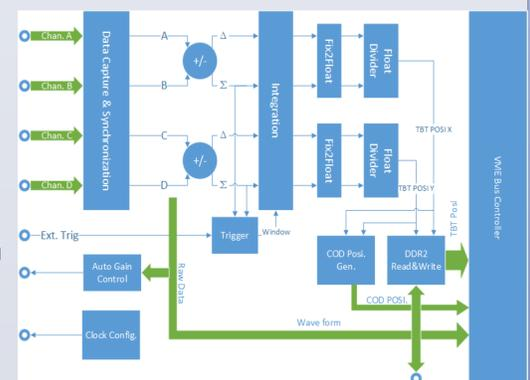
Fig.7: The architecture of the firmware in FPGA
