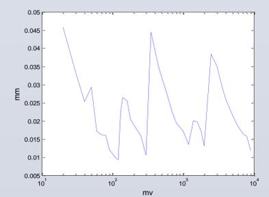
Fig.9: Closed Orbit position resolution
