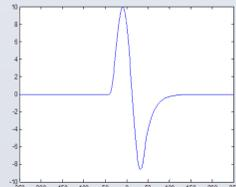
Fig.2-2: Pick-up signal in extraction stage
