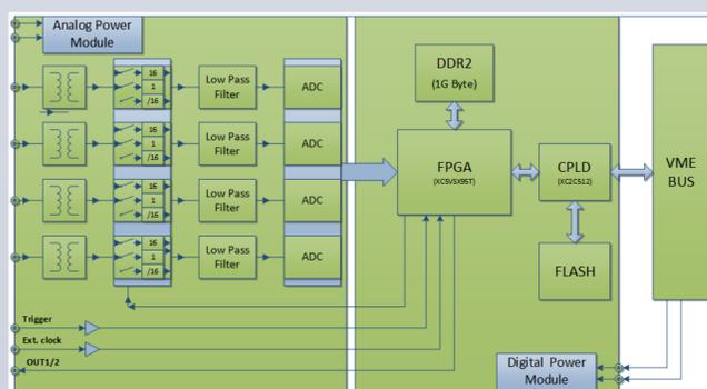
Fig.3: Architecture of CSNS RCS BPM electronics
