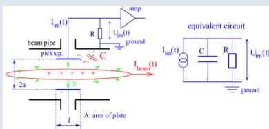
Fig.1: scheme of pick-up electrode and its equivalent circuit
