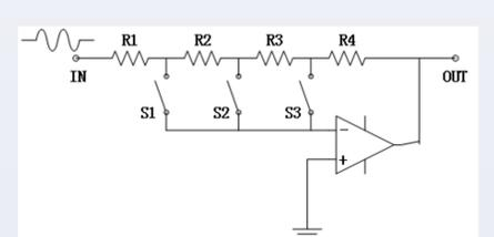
Fig.6: Structure of the second stage amplifier
