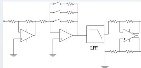
Fig.5: Structure of analog circuit
