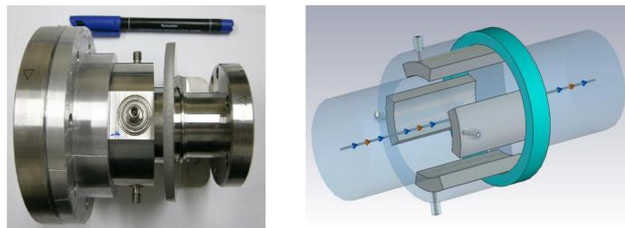
CLIC Drive Beam Stripline BPM Prototype with shortened electrodes
