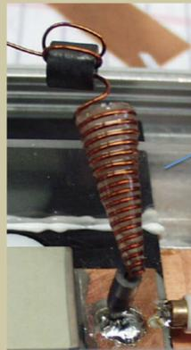
Helical coil and toroid isolating
