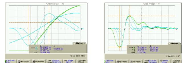
➤ The flat electrode steepness is 1.35, the button electrode steepness is 0.71, the ratio is 1.9.
