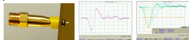
The probe output is proportional to derivative. We integrated not the output but the beam. For probe the beam was a step (12ps), for electrode output the beam was a pulse (18ps) obtained with a differentiator. In the plot above: the electrode output with pulse is blue, the same signal with step and probe is red.
