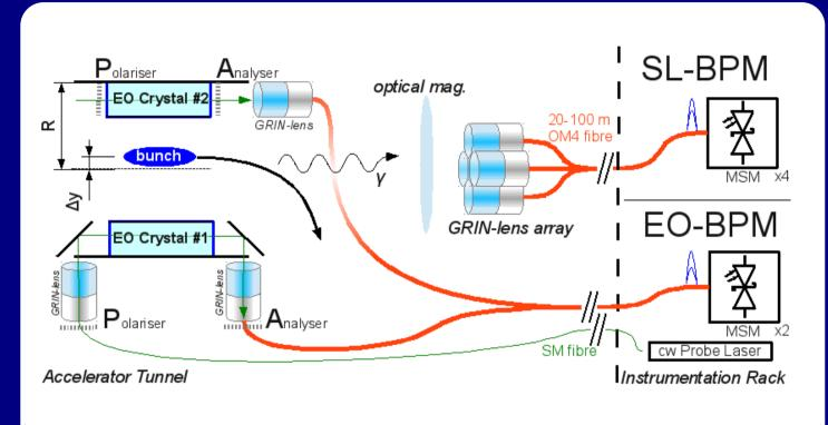
Fibre-coupled MSM-PDs being studied as an back-end option for: A)Electro-Optical-BPM (EO-BPM), & B)Synchrotron-Light-BPM (SL-BPM) aiming at transverse and longitudinal intrabunch beam diagnostics to study ultra-fast intra-bunch head-tail instabilities up to about ~13 GHz → talk: TUBL3
