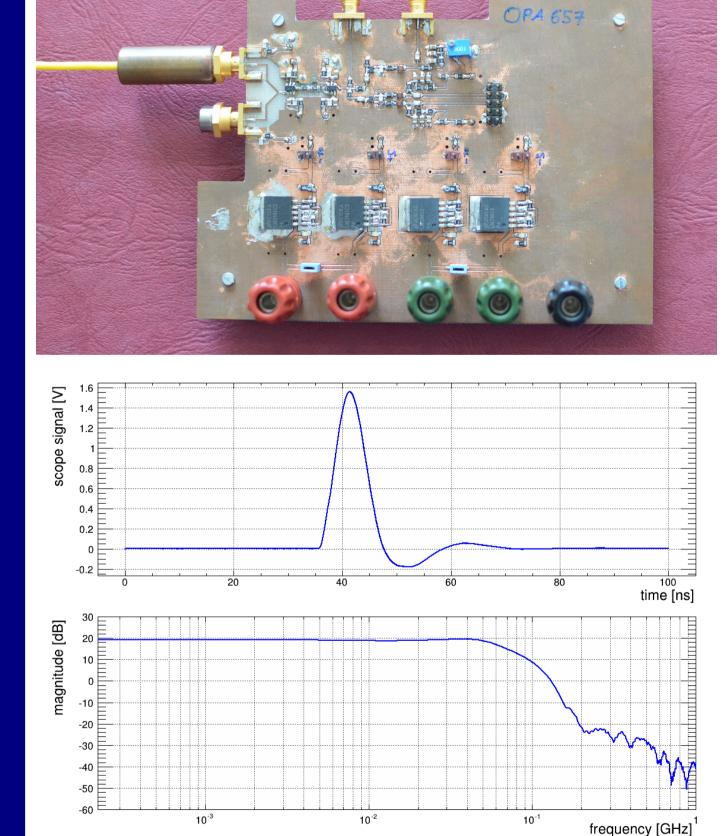
Reduced bandwidth to 80 MHz in favour of higher transconductance  $R_{\downarrow}=25 \text{ k}\Omega$  for sensitivity tests ( $P_{in}$  < 100  $\mu$ W, from initially R<sub>f</sub>=500  $\Omega$ @≈700 MHz).
