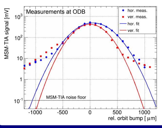
Measured large spot size dominated by chromatic aberrations as the full visible spectrum was taken into account to maximise the incident light power.
