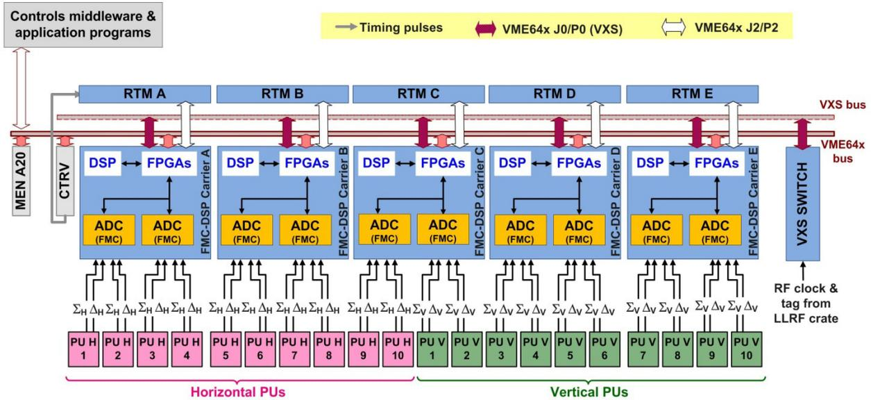
Figure 2: Beam orbit and longitudinal parameters measurement system. Keys: **ADC** - Analogue-to-Digital FMC board; **RTM** - Rear Transition Module; **CTRV** - Timing Receiver Module; **Men A20** – master VME board; **PU H** – Horizontal transverse Pick-Up; **PU V** – Vertical transverse Pick-Up.
