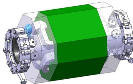
Figure 4: PU assembly inside a quadrupole.
