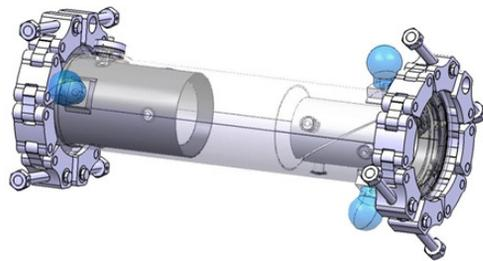
Figure 3: PU assembly inside a dipole.
