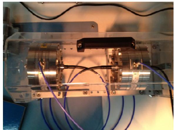
Figure 1: Two FCTs assembly on the test bench.
