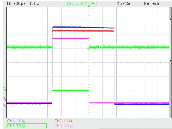
Figure 6: Output signals, ACCT1 (blue), ACCT2 (red), PXI-Out (green) and OE (purple).
