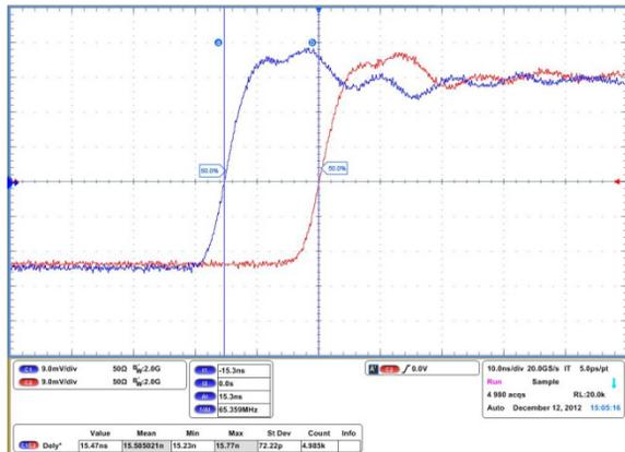
Figure 2: FCTs TOF for un-bunched pulsed current.
