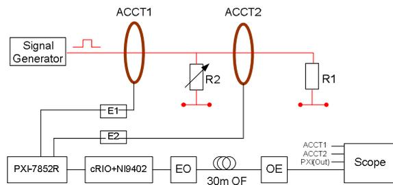
Figure 4: Schematic of laboratory test bench set up.
