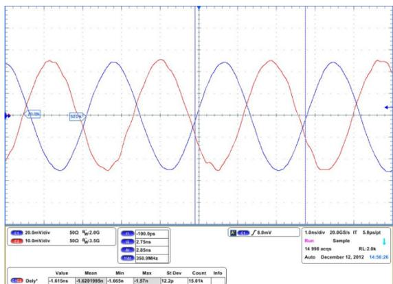
Figure 3: Timing jitter measurement for FCTs rf signal.
