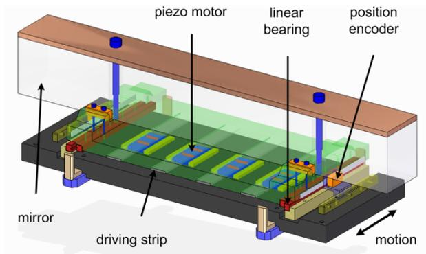
Figure 6: Motor test site with 4 piezo motors. [1]
