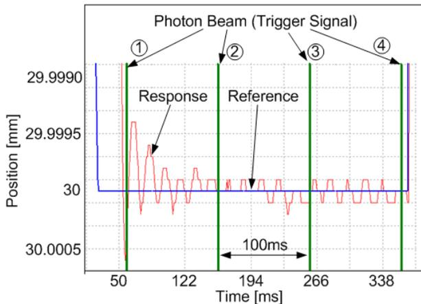
Figure 4: Positional misalignment ( $f = 1$  Hz).
