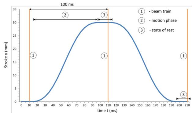
Figure 1: Ideal motion scheme of the mirror at 5 Hz.
