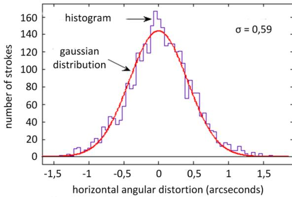
Figure 3: Horizontal angular distortion ( $f = 1$  Hz).
