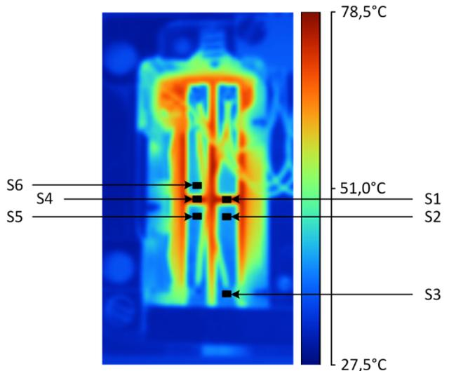
Figure 9: Thermal image of one of the piezo motors with PT100 sensor positions. [4]
