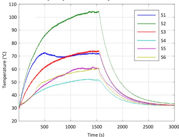
Figure 12: Sensor temperatures under vacuum conditions with mounted covering plate.
