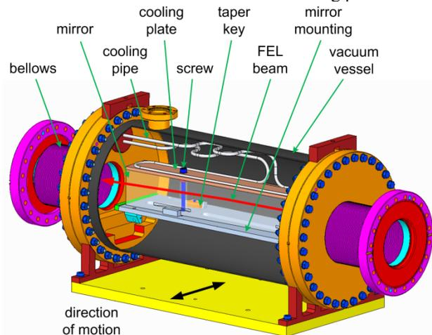
Figure 2: Initial vessel design (3D-CAD-model). [1]
