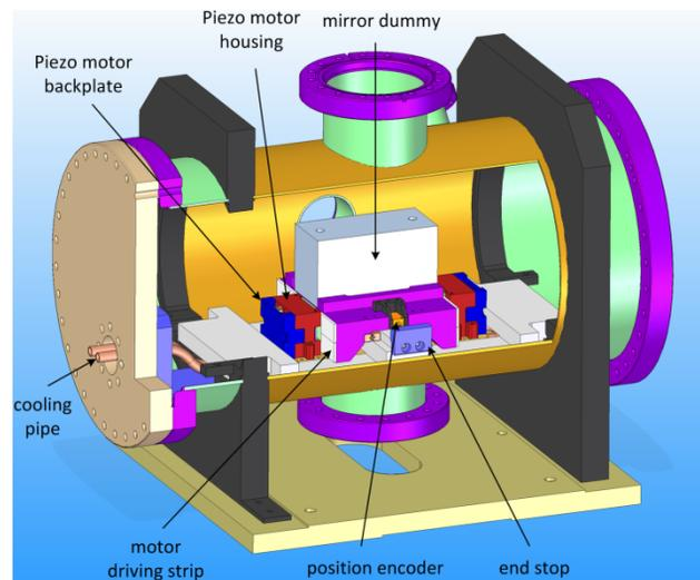
Figure 13: Proposed temperature test setup. [1]
