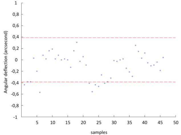
Figure 5: Angular deflection at 5 Hz.
