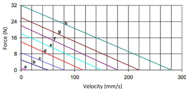
Figure 8: Force vs. velocity diagram of HR8 motor. [3]
