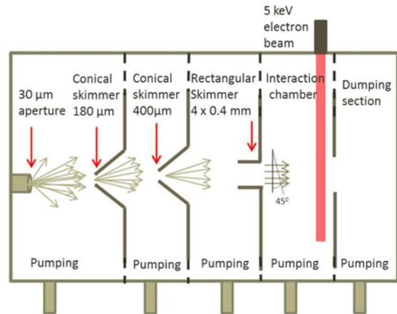
Figure 1: Illustration of the gas jet setup.
