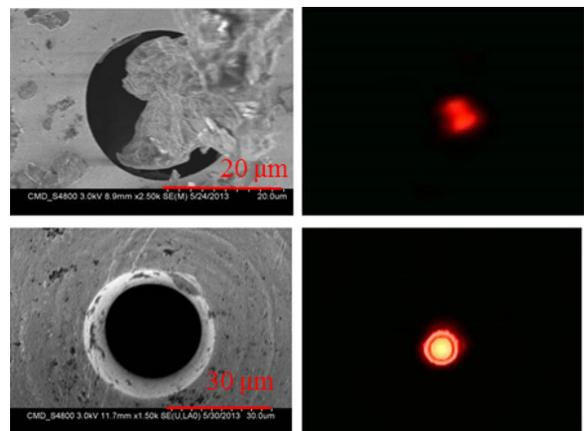
Figure 5: Upper row: orifice blocked; Lower row: orifice is cleaned.
