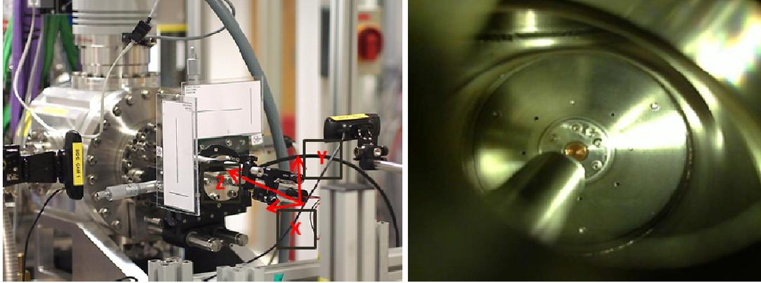
Figure 2: Left: translating stage with 2 cameras for X and Y plane, right: image from the interior of the first vacuum chamber, nozzle's tube and first skimmer can be seen.
