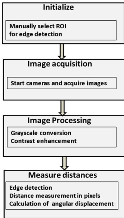
Figure 4: Labview algorithm flowchart.
