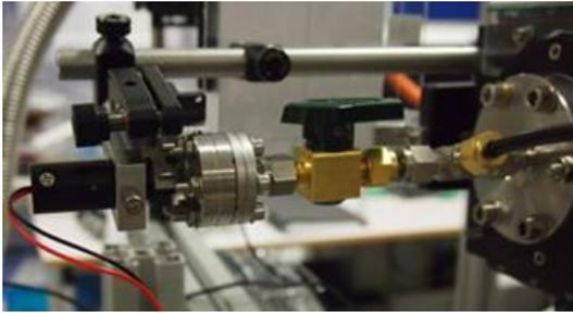
Figure 6 : Photograph of modified gas inlet section.
