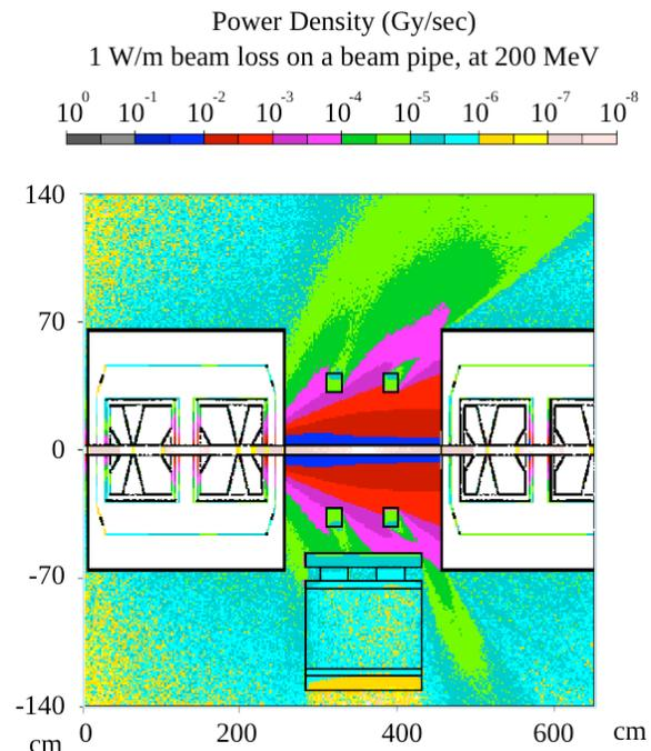
Figure 1: Power density, in Gy/sec, for 1 W/m distributed beam loss on a beam pipe, at 200 MeV.
