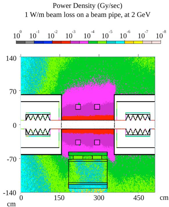
Figure 2: Power density, in Gy/sec, for 1 W/m distributed beam loss on a beam pipe, at 2 GeV.
