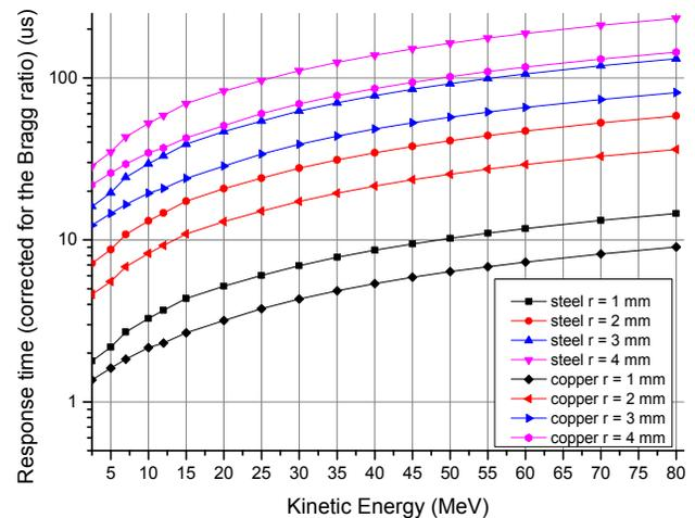
Figure 3: Desired time response (in  $\mu\text{s}$ ) for ionization chambers at different beam energies in the range of 5 MeV – 80 MeV.
