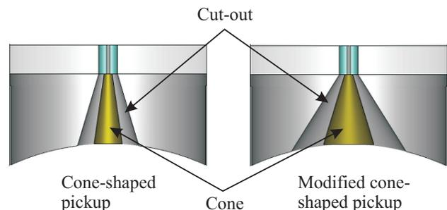
Figure 1: Cross section of the cone-shaped pickup (left) and the modified cone-shaped pickup for high peak-to-peak voltage (right).
