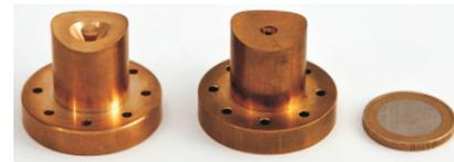
Figure 6: Top: Comparison between the pickup measurements of the nonhermetic prototypes for FLASH and the modified cone pickups. Bottom: Photo of the nonhermetic pickups.
