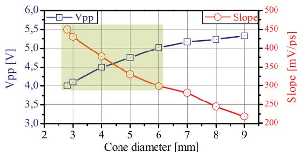
Figure 2:  $V_{pp}$  and the slope at the first zero-crossing as a function of the cone diameter. The optimum area is shaded.
