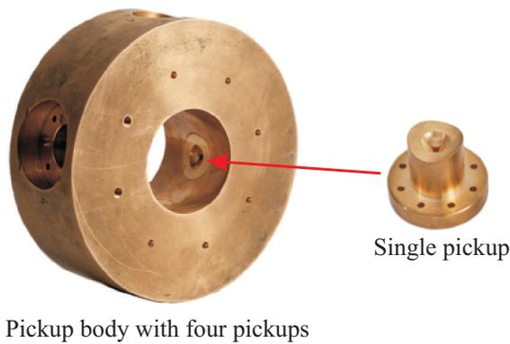
Figure 4: Photo of the nonhermetic prototype. Four pickups are integrated in the body.
