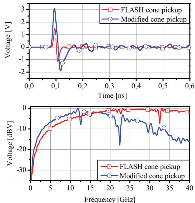
Figure 3: CST PARTICLE STUDIO® simulation of the cone-shaped pickup installed at FLASH and the modified version of the pickup for higher  $V_{pp}$ . Voltage signal in time domain (top), Voltage signal power spectral density (bottom).
