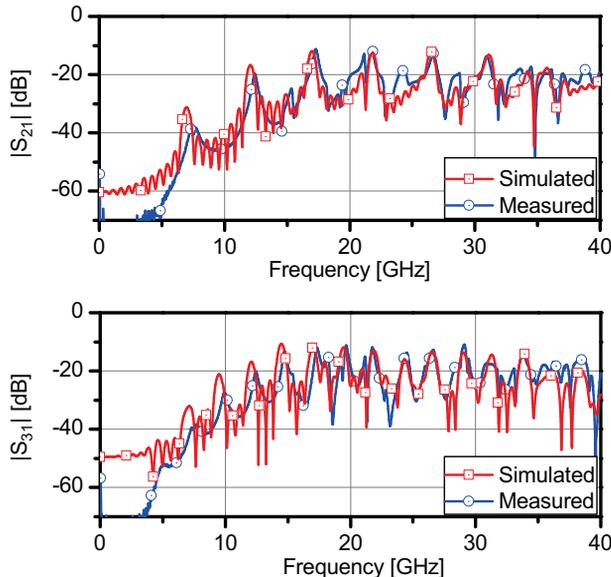
Figure 5: Comparison between simulation and measurements. Top: Between the neighboring pickups. Bottom: Between the opposite pickups.
