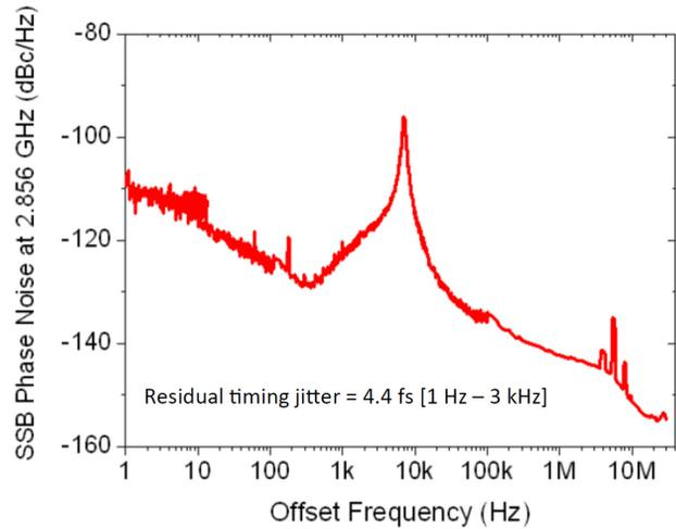
Figure 4: Residual phase noise measurement in the synchronization of RMO and VCO.
