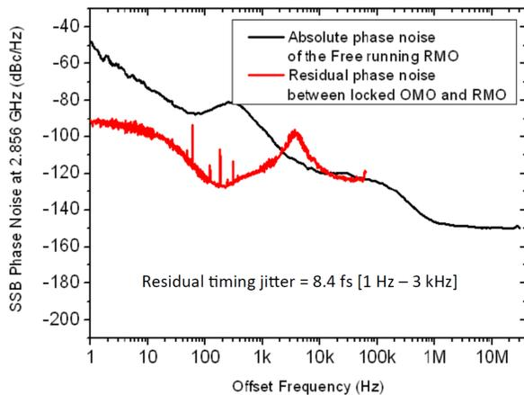
Figure 3: Phase noise measurement in the synchronization of RMO and OMO.
