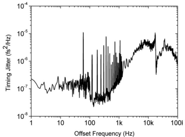
Figure 5: Timing jitter measurement of 610 m optical link.
