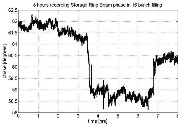
Figure 7: Recordings of Storage Ring phase evolution over an 8 hour period (16 bunch filling).
