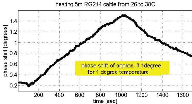
Figure 6: The curve shows the rise and decay of phase shift of 1.3degrees for a 12C differential temperature.
