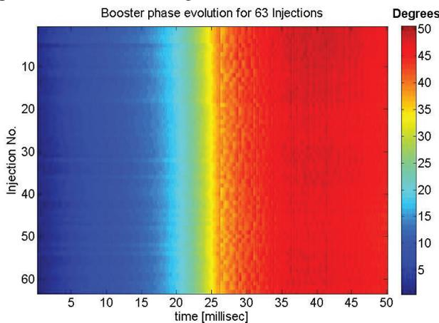
Figure 4a: Phase evolution of the Booster beam during its acceleration cycle for 63 consecutive shots.
