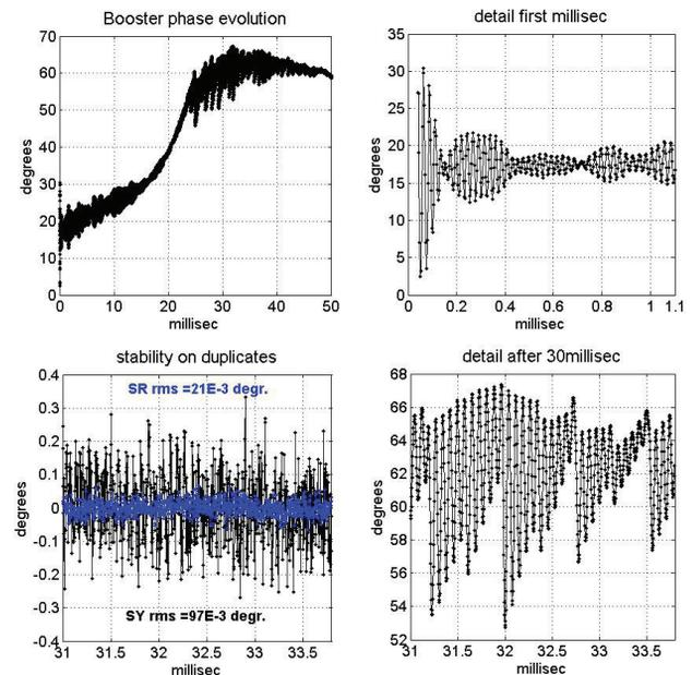
Figure 3: Phase evolution and oscillations of the Booster beam during its 50millisec acceleration cycle.
