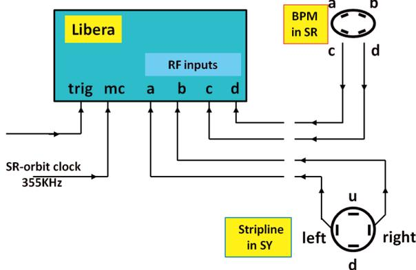
Figure 2: The hardware and interconnections of the phase measurement system between the Storage Ring (SR) and the Booster Synchrotron (SY).
