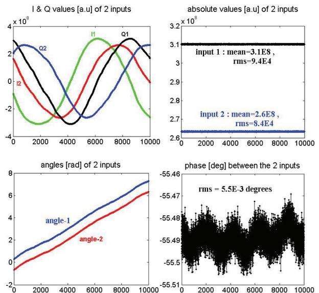
Figure 1: The I and Q values of two RF signals in a single unit (upper-left) and the final differential phase values (lower-right), over a ~2sec recording at 5.5KHz.
