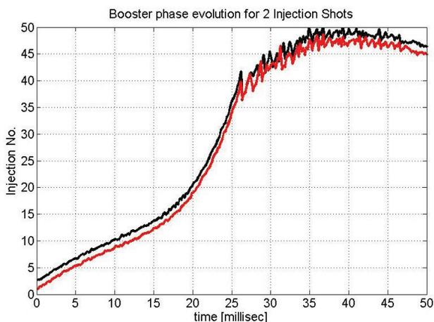
Figure 4b: Phase evolution during the acceleration cycle, for first (black) and last (red) injection of a refill.
