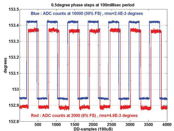
Figure 5: Recordings of phase modulation introduced by an electronically controlled phase shifter.
