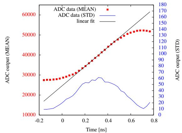
Figure 5: Measurement of the clock jitter contribution during a phase sweep with 1 ns range.
