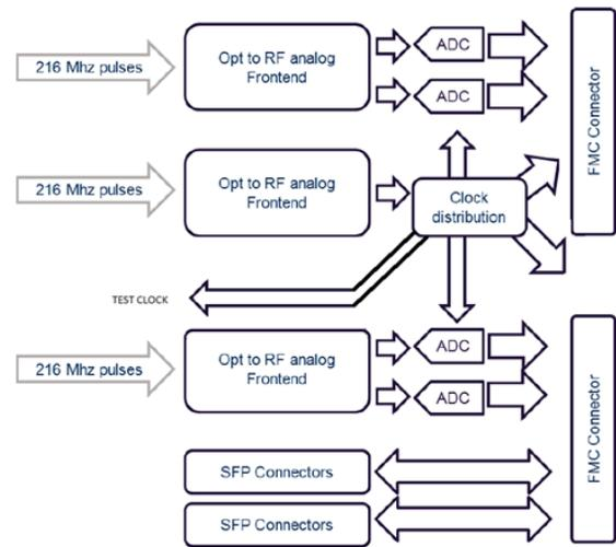
Figure 3: FMC mezzanine card block diagram.
