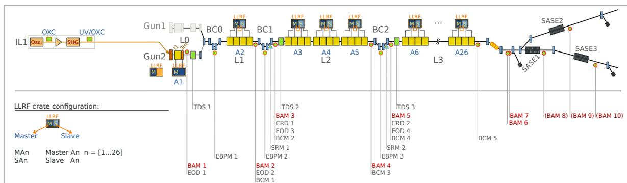
Figure 1: Schematic of the European XFEL with locations of the longitudinal diagnostics. Besides the BAMs, there are also: bunch compression monitor (BCM), energy beam position monitor (EBPM), electro-optical diagnostics (EOD), transverse deflecting structure (TDS), coherent radiation diagnostics (CRD) and synchrotron radiation monitor (SRM).
