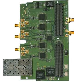
(b) Prototype dual FMC mezzanine card.
