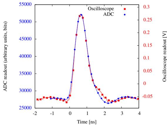
Figure 4: The plot shows the mean values from 1024 subsequent laser pulses measured with the oscilloscope and on-board ADCs.
