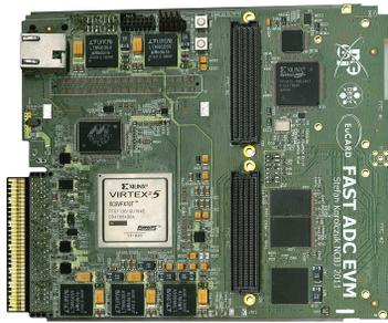
(a) Prototype FPGA based dual FMC carrier board.
