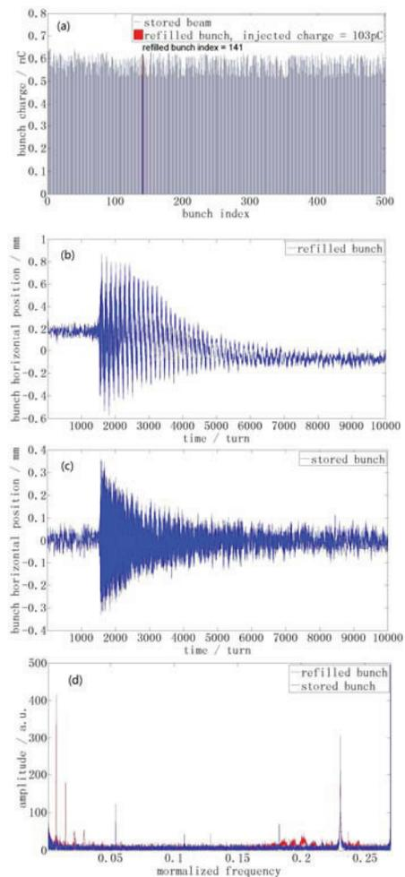
Figure 4: A set of bunch by bunch measurements during injection.
