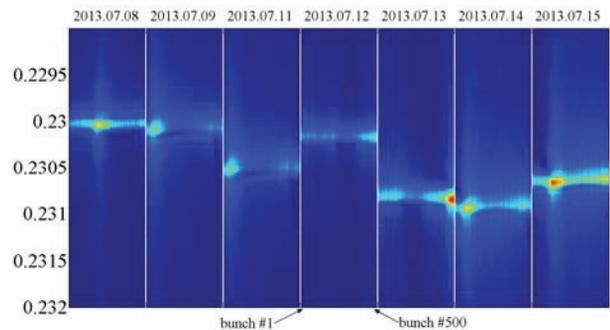
Figure 8: Waterfall displays of horizontal position spectrum during injection in a week.
