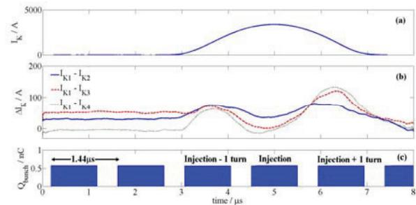
Figure 2: Measured current waveform of injection kickers.
