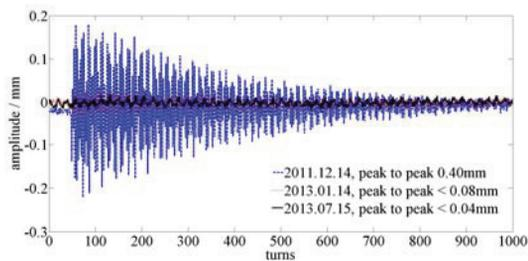
Figure 6: Measured vertical orbit oscillation by injection kick, which reflects the tilts error of kickers.
