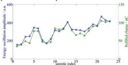
Figure 7: Energy oscillation amplitude of refilled bunch and corresponding refilled charge.
