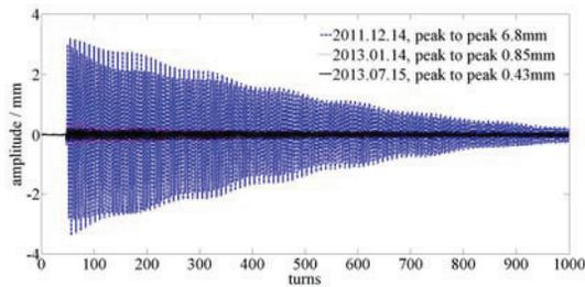
Figure 5: Measured horizontal orbit oscillation by injection kick, which reflects the amplitude and phase mismatch of kicker current waveforms.
