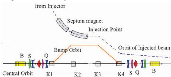
Figure 1: Layout of SSRF ring injection system.
