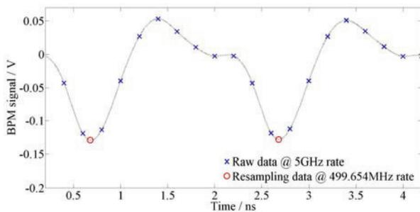
Figure 3: Raw data acquired by digital oscilloscope and virtual re-sampled data using 3rd order spline interpolation method.
