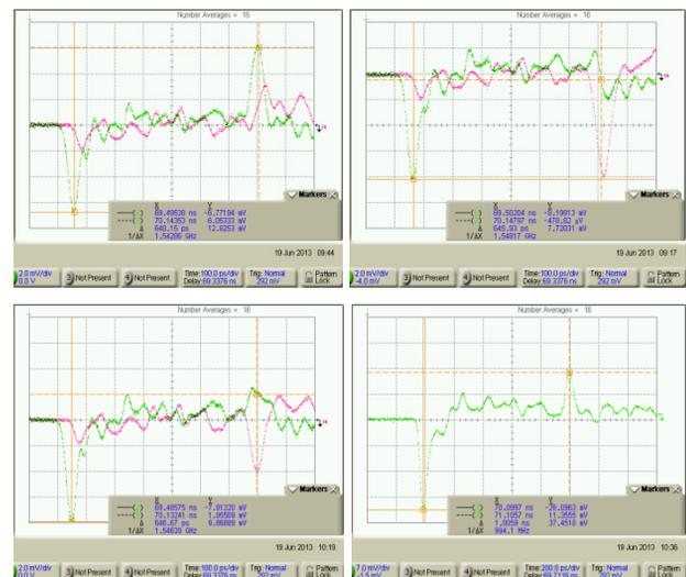
Figure 6: Top left/right: One-gap electrode end is short/open. Bottom left: The end is connected to pin. For these three plots 100ps/div and 2mV/div. Bottom right: Electrode output signal, 200ps/div and 7mV/div.
