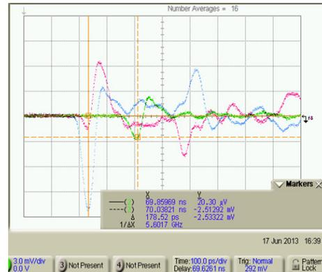
Figure 7: Two-gap electrode, packets in gaps and the output (divided by 2), 100ps/div and 3mV/div.
