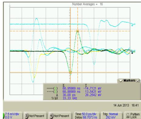
Figure 3: Signals of inductive probe, 50ps/div.
