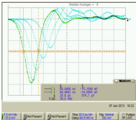
Figure 5: Magnitude and arrival time of the bunch electric field measured at the gap front edge, 20ps/div and 5mV/div.
