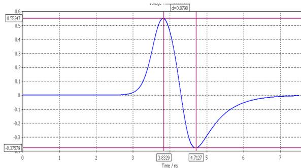
Figure 2 : CST simulated Response of a BPM electrode with CST to a square beam input of 1 ns duration.
