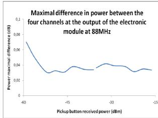
Figure 4: Maximum power difference between the four inputs at 88 MHz.
