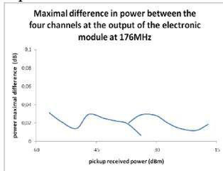
Figure 6: Maximum power difference between the four inputs at 176 MHz.
