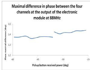
Figure 5: Maximum phase difference between the four channels at 88 MHz.
