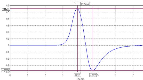
Figure 2 : CST simulated Response of a BPM electrode with CST to a square beam input of 1 ns duration.
