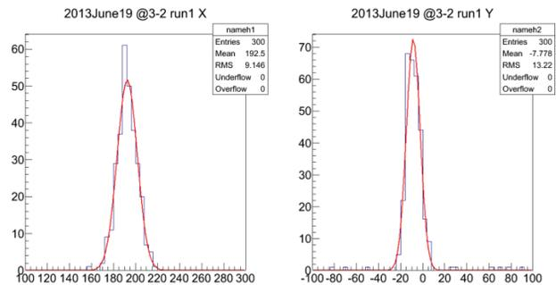
Figure 8: Position histogram example of beam test (0.3 nC). X-axis is position in  $\mu m$ .
