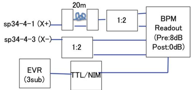
Figure 7: Beam test setup of BPM readout system.
