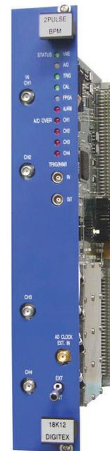
Figure 1: Photograph of BPM Readout System Board.
