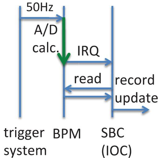
Figure 5: Timing diagram of BPM readout system.
