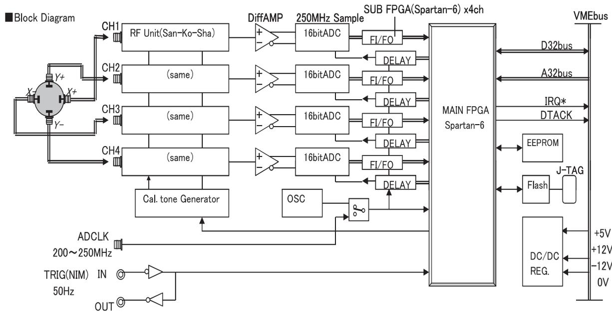
Figure 2: Block diagram of the BPM readout system.
