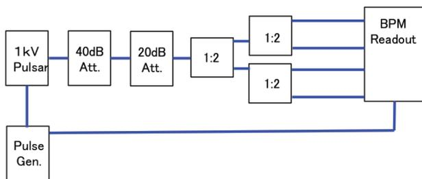
Figure 6: Pulsar Test setup of BPM readout system.
