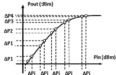
Figure 5: Main idea of the linearity test setup. It is possible to determine the linearity of the response of an RF device by measuring the difference in the output power for a known difference in the input power. If the difference between adjacent points on the output power remains constant, this determines the range of input power within which the system is linear.
