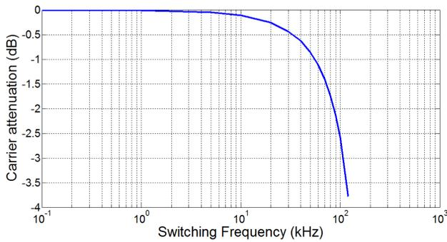
Figure 3: Switching speed effect on the RF signal attenuation. The switches used in the test have 2  $\mu$ s stabilization time (10 - 90 % specification).
