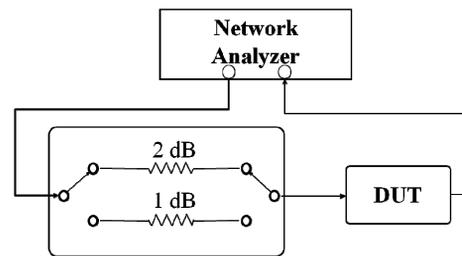
Figure 4: Block diagram of the setup used for measuring nonlinearity of RF electronics.
