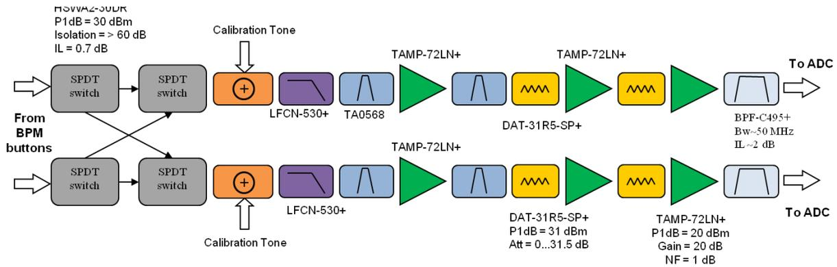
Figure 2: RF chain developed for the SIRIUS RF Front-End of the BPM electronics. Only one pair of channels is shown since the electronics is symmetric.
