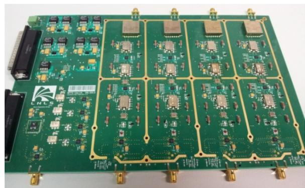
Figure 1: RFFE board. Ten layers of the Rogers RO4350 RF substrate.
