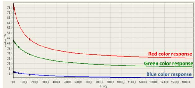
Figure 5: Calibration curves: amplitudes of the red, green and blue colours in function of the dose. For their better sensitivity only red and green can be used for dose measurement.
