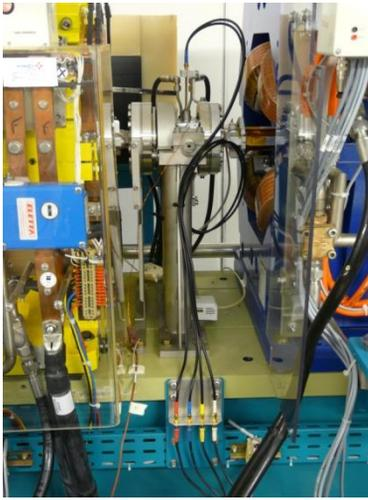
Figure 4: Insertion of disposable pigtails between BPM and its cables to avoid damages of the long and expensive cables.
