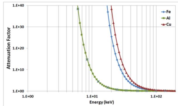
Figure 12: Attenuation factor applied to X-rays crossing 3 mm of Al (green), Fe (blue) or Cu (red) depending on their energy.
