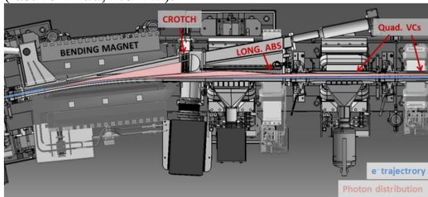
Figure 8: Photons produced in the dipole magnets are absorbed by one of the following elements depending on their emission angle: crotch, longitudinal absorber or quadrupole VC (top view).
