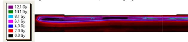
Figure 7: Dose distribution measured longitudinally on the surface of one of the quadrupole VC. Scanned image has been converted in dose scale.
