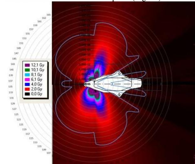
Figure 10: Correlation between the dose distribution measured with Gafchromic films and the calculation of 15 keV X-ray transmission factor (blue curve) as a function of the crossed Al thickness (transversal plane).
