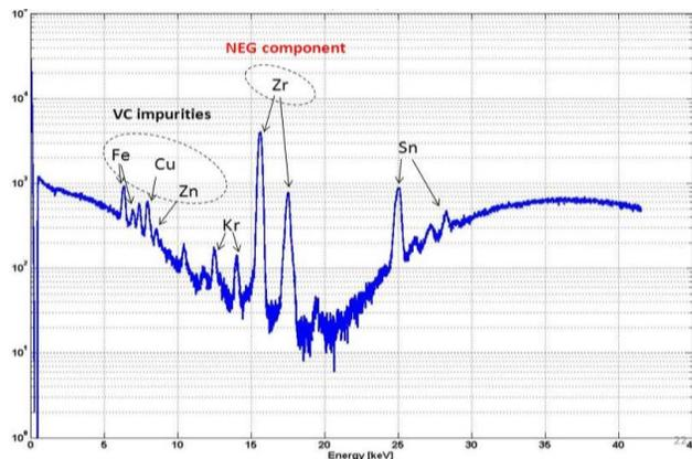
Figure 11: X-ray spectrum analysis acquired with a silicon drift detector. Measurement confirms the fluorescence of NEG coating material (Zr) and of some impurities in the Aluminium of the VC (Fe, Cu and Zn).
