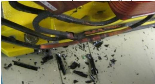
Figure 1: Insulating layer of some sextupole magnets has become brittle due to radiation.
