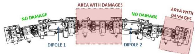
Figure 3: Example of damaged area for one cell of the SOLEIL storage ring. Damages are located around the so-called “quadrupole vacuum chambers” installed downstream dipole magnets.
