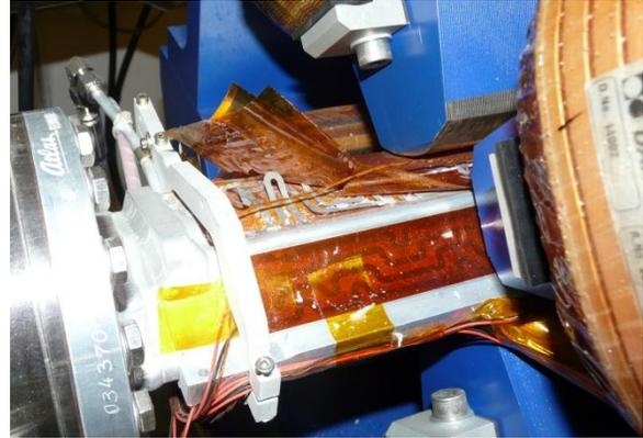
Figure 2: Glue that sticks together different kapton foils of some baking out films is damaged by radiation.
