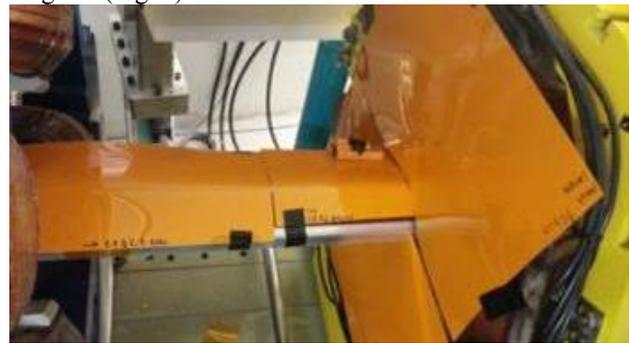
Figure 6: Gafchromic films installed on the VC and against a sextupole magnet in cell C08 (before exposition).
