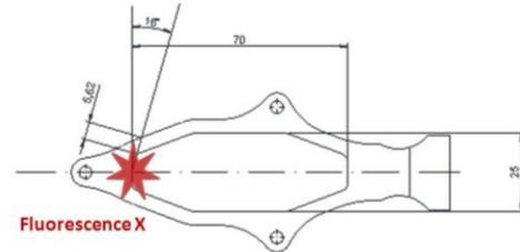
Figure 9: Cross section of a quadrupole VC. Minimum thickness is 3 mm. Upstream dipole synchrotron radiation is intercepted by the chamber inducing X-ray fluorescence of its materials.
