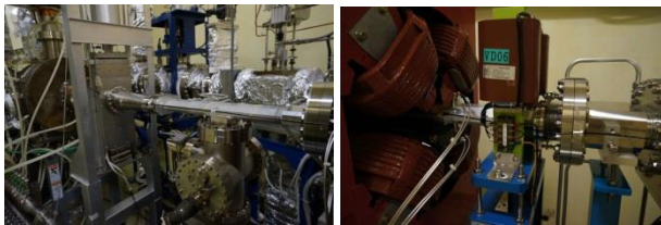
Figure 5: Black cables mounted on the side of the vacuum chamber are the optical fibers for the loss monitor. The fibers can be fed through the magnet due to the non-magnetic nature of the medium.
