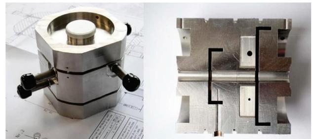
Figure 5: Steel S-band cavity BPM for E-XFEL.
