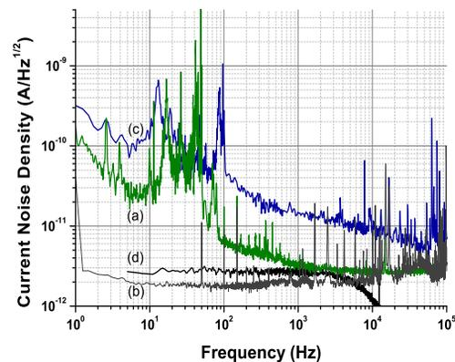
Figure 3: The figure above shows the measured current noise density of the improved FAIR-CCC with Nanoperm M764 core (a) whereas plot (b) represents the intrinsic current noise density of the Supracon SQUID sensor CP2 blue. For comparison the measured current noise density of the DESY-CCC pick-up coil including a Vitrovac 6025F core is shown (c) whereas plot (d) represents the intrinsic current noise density of the SQUID sensor UJ111 from Jena University.
