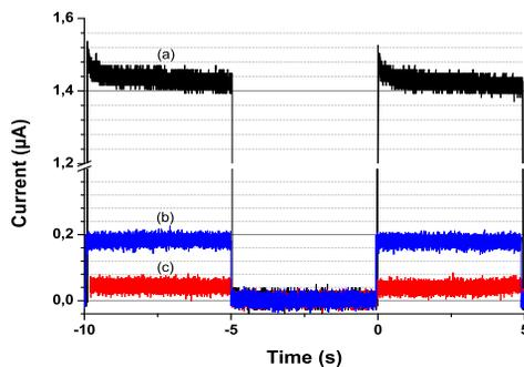
Figure 4: Full-bandwidth response of the FAIR-CCC to a rectangular current signal of 1.438  $\mu\text{A}$  (a), 185 nA (b), and 42.5 nA (c) applied to the additional calibrating loop.
