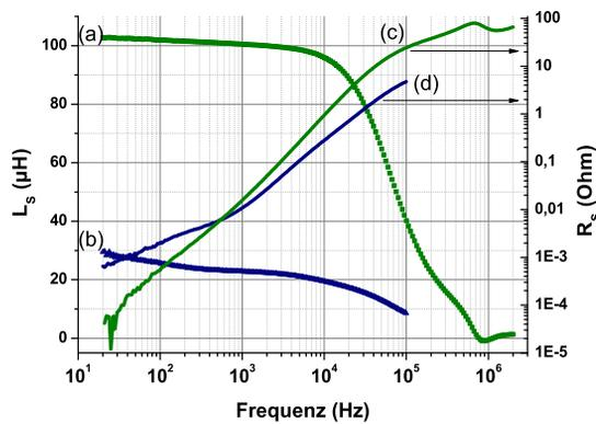
Figure 2: Comparison  $L_S$  ( $\nu$ ) and  $R_S$  ( $\nu$ ) of the welded pick-up coil with Nanoperm M-764-01 core ((a) and (c)) and the DESY-CCC pick-up coil with Vitrovac 6025F core ((b) and (d)) 4.2 K.
