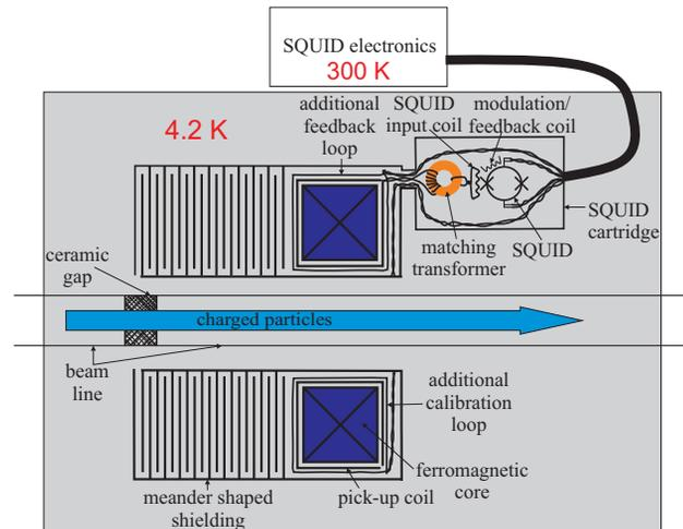
Figure 1: Circuit diagram of the CCC.
