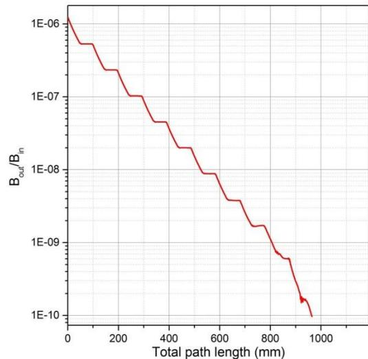
Figure 4: Field attenuation through a meander shaped magnetic shield geometry. The attenuation is plotted against the total path the field has to propagate through the shield geometry.
