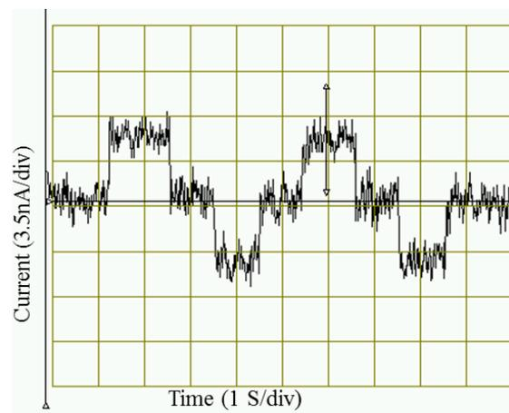
Figure 7: 5 nA peak to peak signal in full bandwidth.
