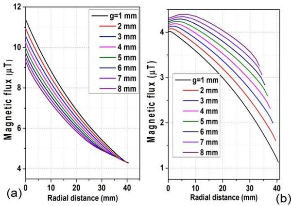
Figure 2: Attenuation of the magnetic field in  $+\vec{r}$  direction (a) and  $-\vec{r}$  direction (b) plotted for various gap widths.
