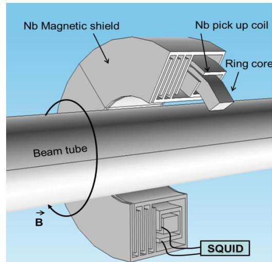
Figure 1: Schematic view of the sensor unit of the CCC system. The complete sensor part is operated at 4.2 K.
