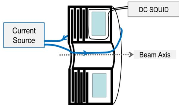
Figure 6: Schematic of the current measurement set up with wire loop wound around the magnetic shield to apply a known current to stimulate beam current. The CCC sensor unit was maintained at 4.2 K during the measurements.
