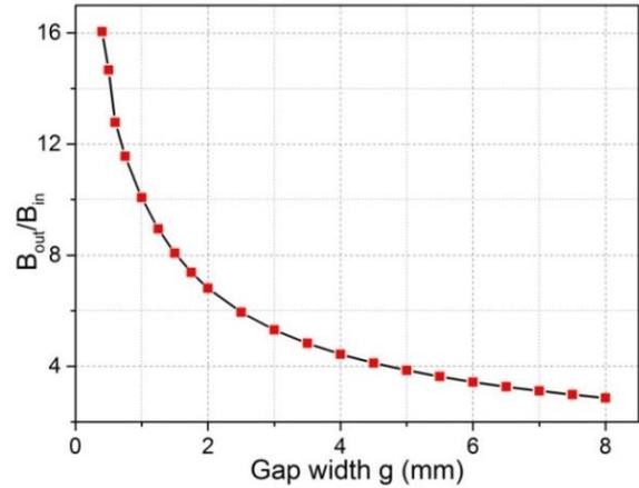
Figure 3: Variation in field attenuation while passing through a single meander curve as a function of gap width,  $g$ .
