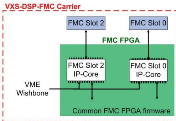
Figure 6: IP-cores instantiation in the FMC FPGA.
