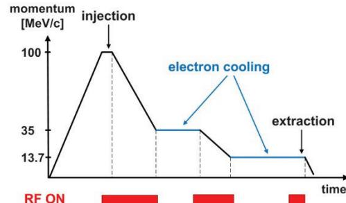
Figure 1: Schematic view of the ELENA cycle.
