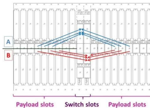
Figure 3: VXS interconnect structure obtained with two Switch boards.
