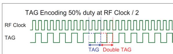
Figure 7: RF clock and TAG encoding.
