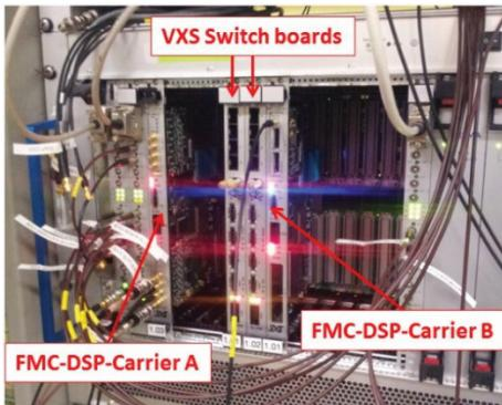
Figure 2: Two-board LLRF test system installed in CERN's PSB during the 2012-2013 run.
