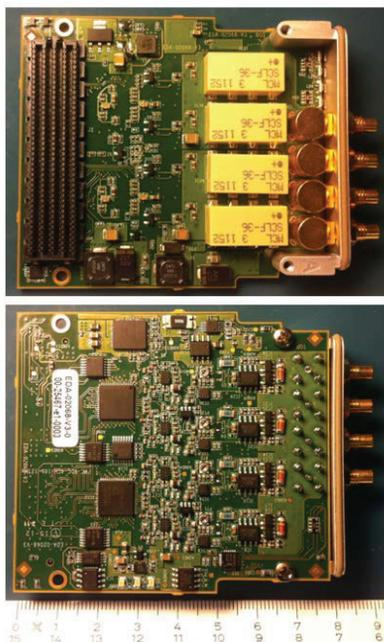
Figure 5: ADC FMC top (above) and bottom (below).
