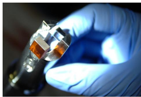
Figure 2: Photograph of an EO GaP crystal, mounted on its support (image courtesy of N. Hiller, KIT).
