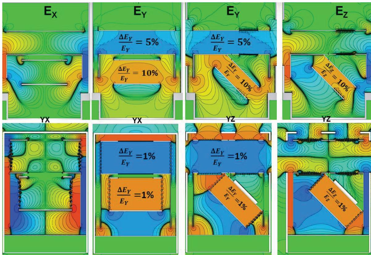
Figure 4: Fields simulation for old BCSM design (top row) and new one (bottom row). X, Y, Z-components of fields are shown in different planes (Z-axis correspond to beam direction). New design provides fields uniformity improvement by an order of magnitude.
