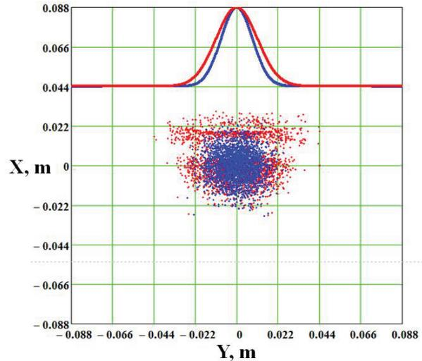
Figure 6: BCS image and profiles simulation for U-70 IHEP. Analyzed beam (blue) with  $1.7 \cdot 10^{13}$  protons per pulse and measured BCS image (red) at 5 kV/cm extracting field. Y-profile spreading is 45%.
