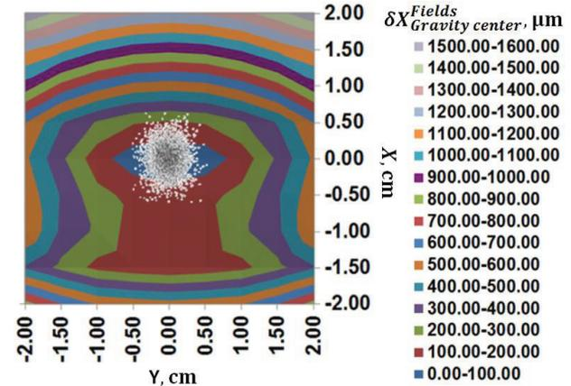
Figure 1: Beam gravity center offset depending on initial coordinates X/Y at slit plane in extracting condenser. Also beam region is shown in the center of this plane.
