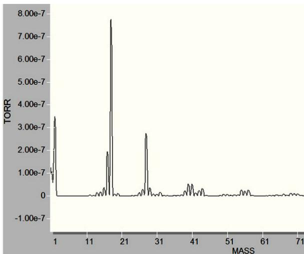
Figure 5: Mass spectrum of residual gas in BCSM region at INR linac. Water vapour dominates.
