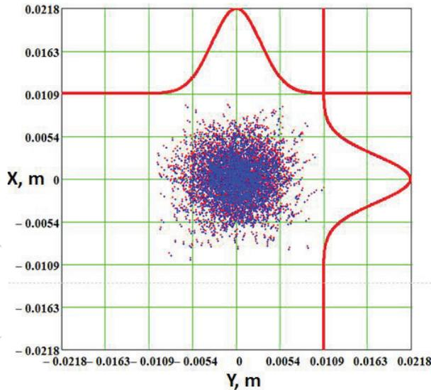
Figure 7: BCS image and profiles simulation for LU-20 NICA JINR. Analysed beam (blue) and measured BCS image (red) at 3 kV/cm extracting field. Relative errors of measurements of rms beam size and position of beam gravity center are  $\sim 1\%$ , and profiles difference is indistinguishable.
