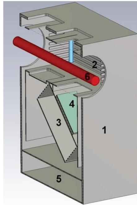
Figure 3: 3D-design of BCSM proposed for NICA. 1 – high vacuum box, 2,3 – extracting and analyzing condensers respectively with correcting electrodes, 4 – electron-optical converter, 5 – forevacuum region for electronics, 6 – analysed beam.
