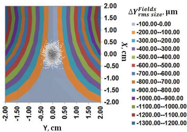
Figure 2: Decreasing of observed rms beam size depending on initial coordinates X/Y at slit plane in extracting condenser. Also beam region is shown in the center of this plane.
