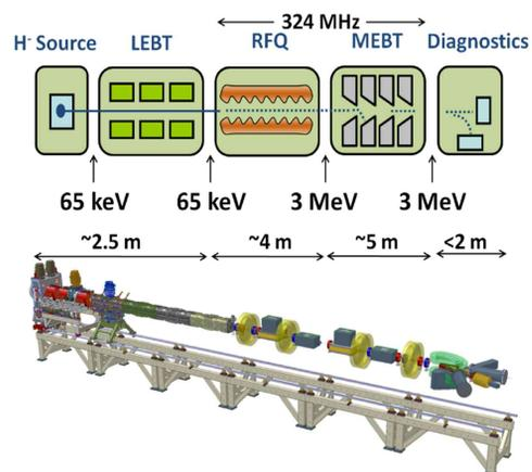
Figure 1: Overview of the FETS beamline components.
