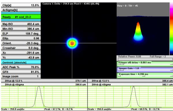
Figure 7: Beam profile close to the focus, after collimating optics, beam expander and  $f = 500$  mm focusing lens.
