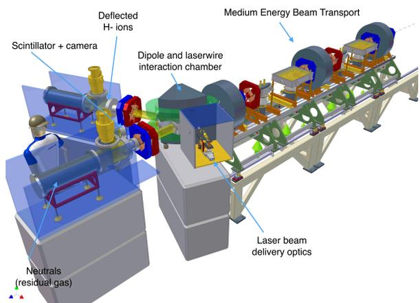
Figure 3: External view of the FETS MEBT and laserwire diagnostic chamber within the dipole magnet.
