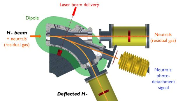
Figure 2: Photodetachment principle in the interaction chamber of the FETS laserwire emittance scanner.
