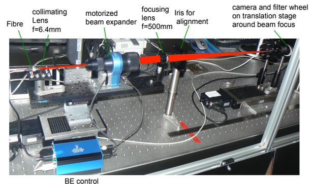
Figure 5: Beam delivery system set up for  $M^2$  measurements.
