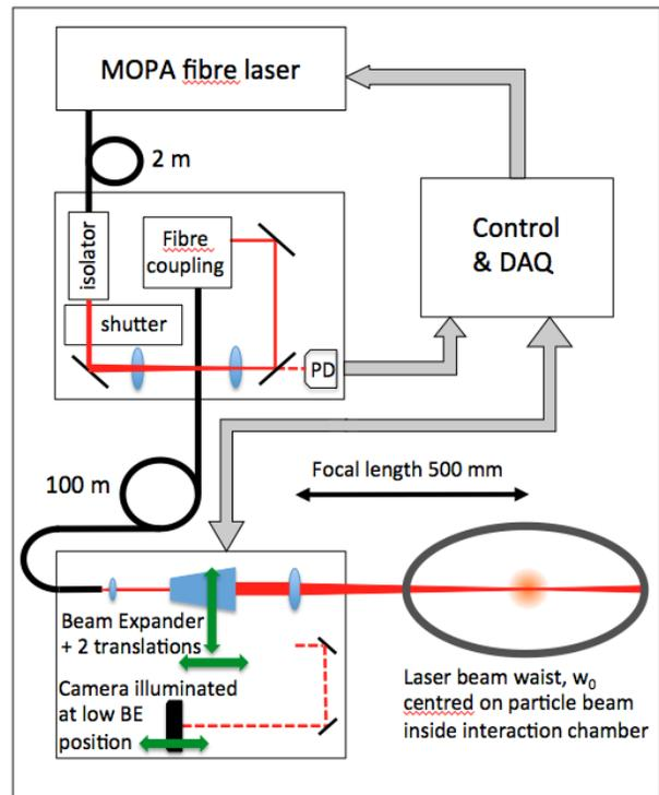
Figure 4: Optical layout of laser transport and beam delivery system.
