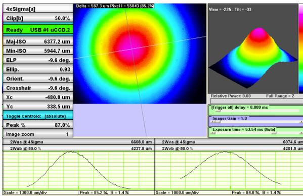
Figure 6: Beam profile directly out of the 100m long transport fibre, with no collimation optics.
