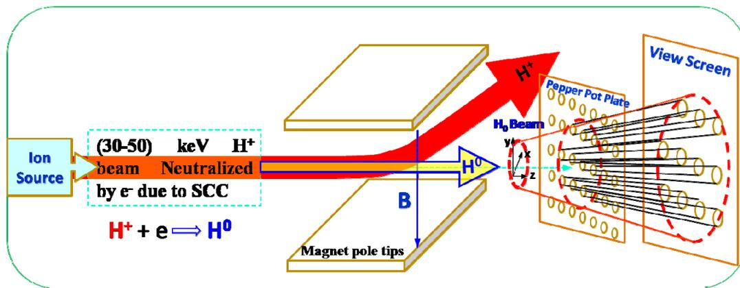
Figure 1: Outline of beam emittance monitor based on neutral beam fluorescence.
