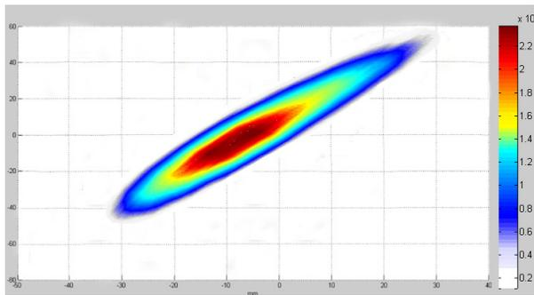
Figure 4: Measured emittance distribution (vertical) using the neutral beam fluorescence based emittance measurement system.
