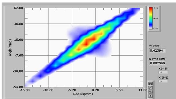
Figure 5: Measured emittance distribution (vertical) using the MSSW emittance monitor.
