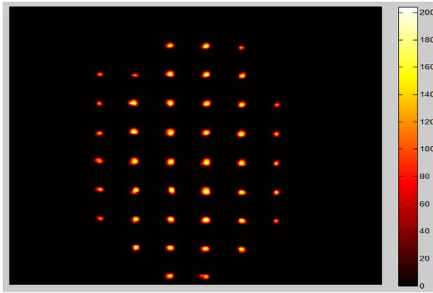
Figure 3: Image of  $H^0$  beamlets on the fluorescence screen.
