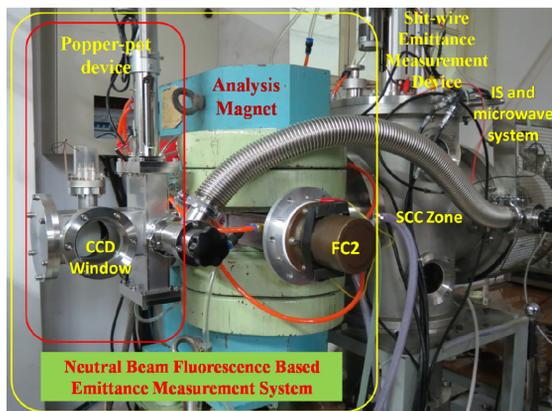
Figure 2: PKU ion source test bench and new emittance measurement system.
