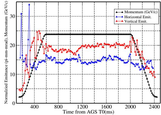
Figure 3: AGS emittance on the up and down ramp with  $2 \times 10^{11}$  intensity. Constant beta function of 22m was used for both vertical and horizontal planes.
