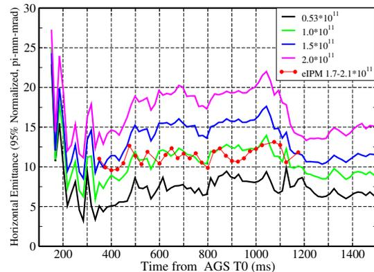
Figure 6: Horizontal emittance in the AGS on the ramp with various intensities. At 1100ms, RF is turned off. The reported emittance is reduced as the space charge force is diminished. The eIPM data was included for comparison. It is seen that the values reported by the eIPM is smaller than IPM (with RF off) by about 1-2pi.
