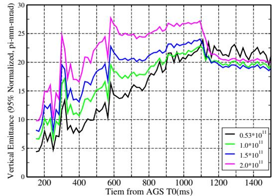
Figure 4: Vertical emittance in the AGS on the ramp with various intensities. At 1100ms, RF is turned off. The reported emittance is reduced as the space charge force is diminished.
