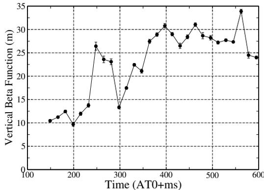
Figure 2: The measured vertical beta function along the AGS ramp. The flattop is reached at 581ms from the AGS T0. Transition is crossed around 300ms.
