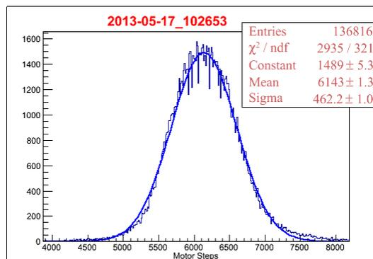
Figure 1: A horizontal beam profile measured by polarimeter. The smooth curve is the Gaussian fit. The horizontal axis is the step count. This particular profile gives beam sigma as 1.02mm. With dispersion contribution subtracted, the normalized emittance is  $12.6\pi$ mm-mrad. Standard beta function 10m is used.
