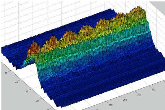
Figure 5: The average TBT profiles for the 300 to 600 turns at AGS injection.
