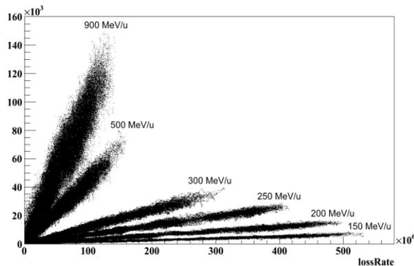
Figure 7: Diagram shows the BLM signal vs. loss rate.
