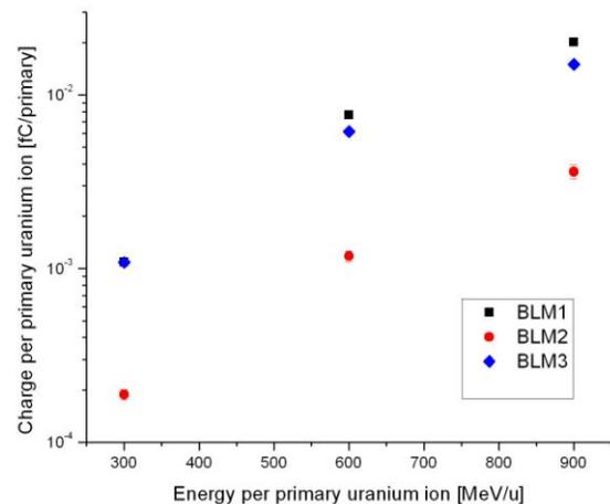
Figure 3: The simulated response function of LHC-type ionization chamber.
