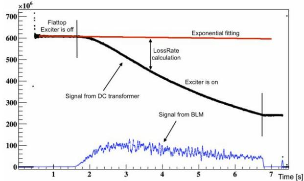
Figure 6: The signals measured by DC transformer and scintillation beam loss monitor.
