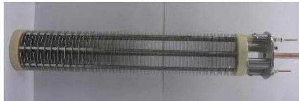
Figure 1: The BLM LHC-type ionization chamber without steel cover [1].
