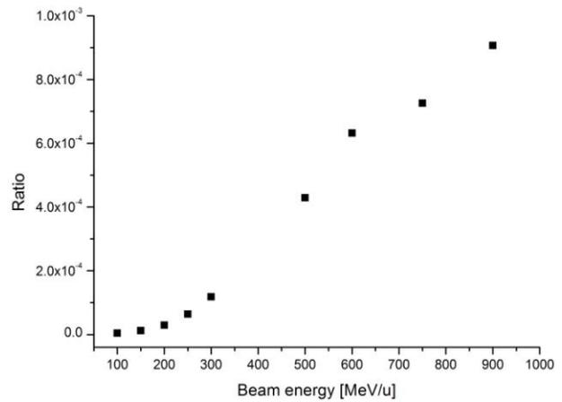
Figure 8: BLM signal to loss rate ratio in dependence on beam energy.
