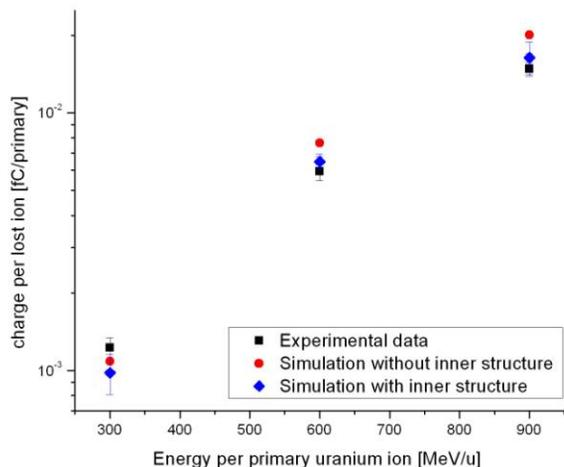
Figure 4: BLMI1 response function of LHC-type ionization chamber. Comparison between experimental data and simulations.
