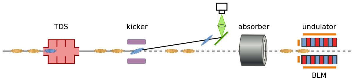
Figure 1: Schematic layout of the longitudinal bunch profile monitor consisting of a TDS, fast kicker magnet, off-axis scintillation screen and imaging system (not to scale). The set-up is located directly upstream of the FEL undulators. Quadrupoles and other components are omitted. The bunch-stealing mode is illustrated with blue (for the measurement) and yellow bunches (for the generation of FEL radiation).
