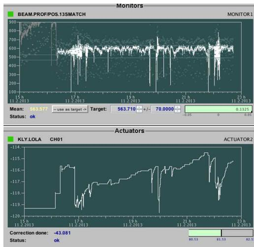
Figure 5: Operator control panel of the slow TDS RF phase feedback showing histories of the centre-of-mass position of the beam image on the imaging screen (top) and TDS RF phase setpoint (bottom).
