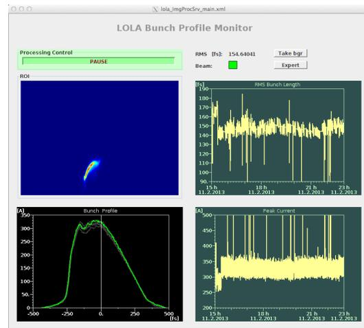
Figure 6: Operator panel for the longitudinal bunch profile monitor: Processed single-shot image (upper left), current profile (lower left), history of bunch length (upper right) and history of peak current (lower right).
