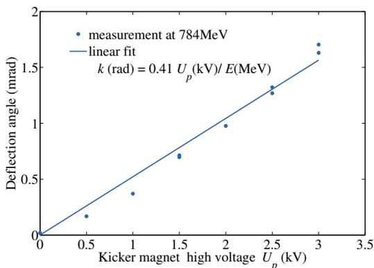
Figure 2: Cross-calibration of the kicker magnet with a corrector magnet for the determination of the kick strength  $k$ .
