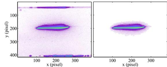
Figure 4: Example of the image processing algorithm with a raw image after background subtraction (left) and the final processed image (right).
