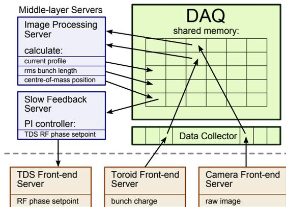
Figure 3: Simplified diagram of the data flow for the longitudinal bunch profile monitor and slow TDS RF phase feedback (for more detail see text).
