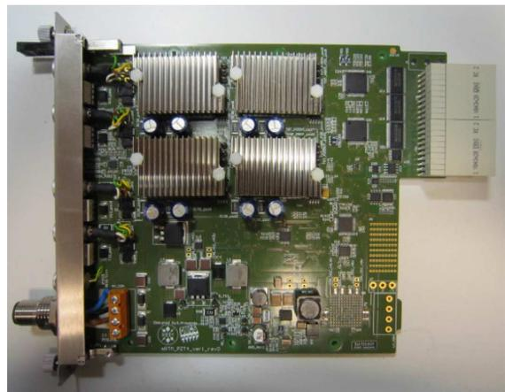
Figure 4: Photograph of the DRTM-PZT4 4-channel piezo driver board.
