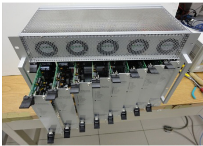
Figure 4: Corrector power supply crate. There are 8 power supply regulation modules in one crate and the most left slot will be plugged in one CPSC.
