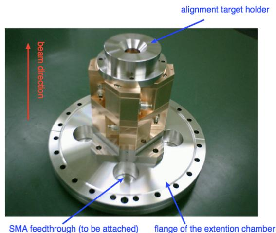
Figure 1: IPBPM assembly as installed at IP area of the ATF2 beam line [8].
