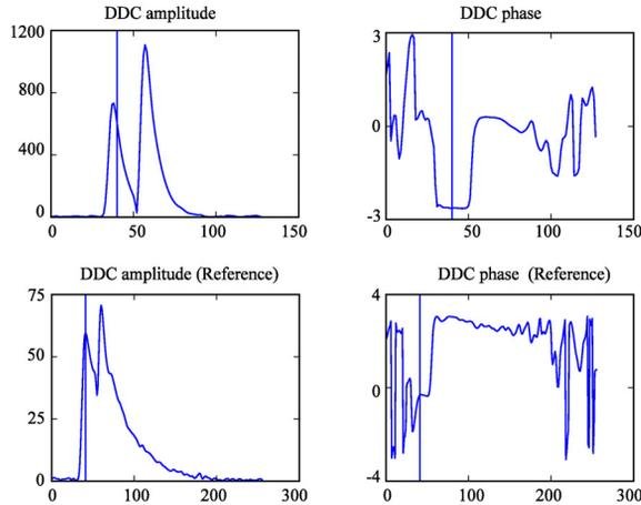
Figure 4: An example of the DDC amplitude and phase of dipole and reference cavity signals. Blue vertical bar is the location for the sampling.
