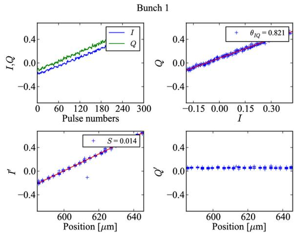
Figure 5: An example of vertical calibration for the first bunch with 10 dB attenuation.
