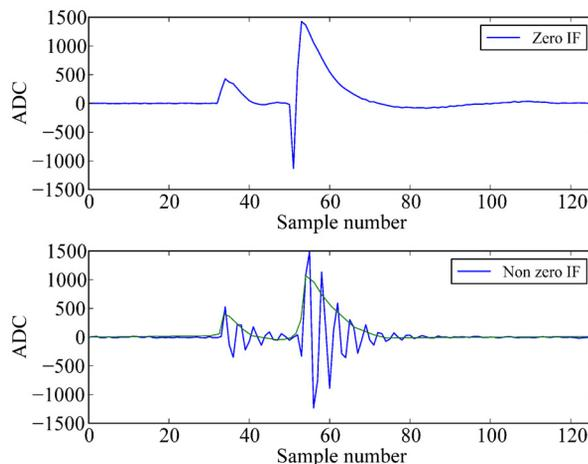
Figure 3: An example of the raw zero and nonzero IF frequency digitised waveforms from the IPBPM electronics in two bunch operation. Green trace is DDC amplitude.
