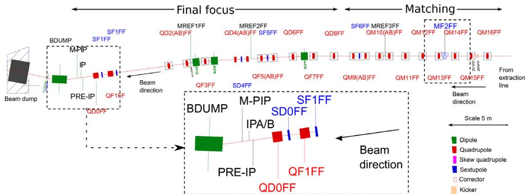
Figure 2: Layout of the ATF2 from the  $\beta$  matching section onwards to the IP and dump. A zoom of the IP region is shown.
