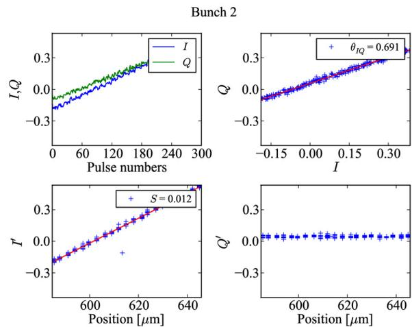
Figure 6: An example of vertical calibration for the second bunch with 10 dB attenuation.
