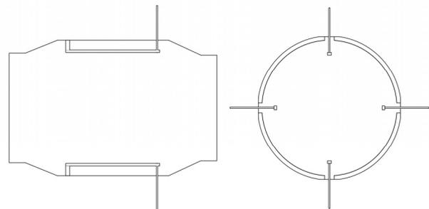
Figure 7: Geometry of the BPM in preparation for the 3-50BT collimator.
