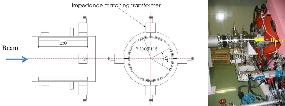
Figure 2: Geometry of the BPM at the 3-50 BT in J-PARC. Left to right, the side view, the cross section and the photograph of the BPM. The load is the impedance matching transformer (15:2) with 50 Ω load.
