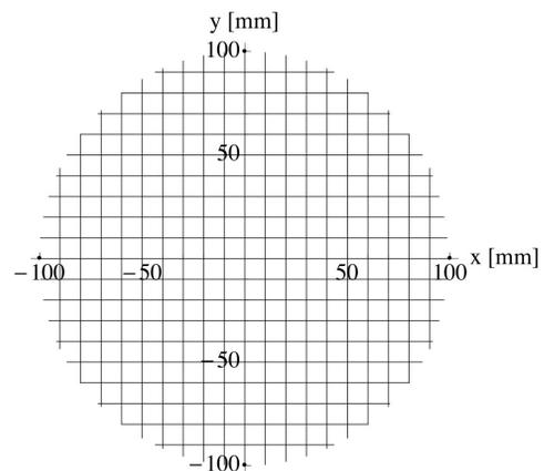
Figure 3: Mapping of the BPM of the 3-50BT. The grid lines represent the beam position, spanning to the BPM aperture with 10 mm interval in the transverse plane.
