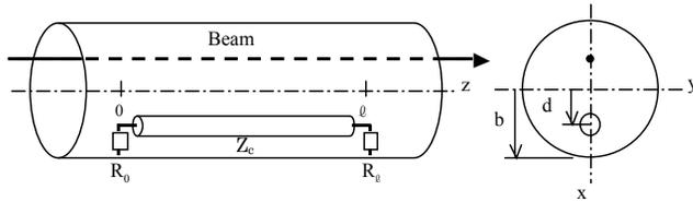
Figure 1: Example: one conductor and a beam.
