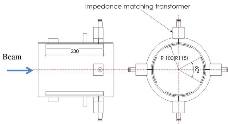
Figure 2: Geometry of the BPM at the 3-50 BT in J-PARC. Left to right, the side view, the cross section and the photograph of the BPM. The load is the impedance matching transformer (15:2) with 50 Ω load.
