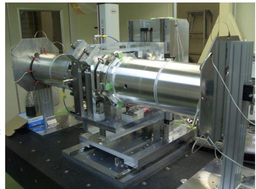
Figure 5: Calibration with stretched-wire method.
