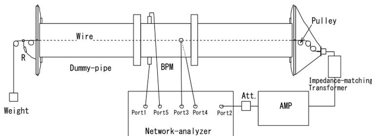
Figure 5: Calibration with stretched-wire method.
