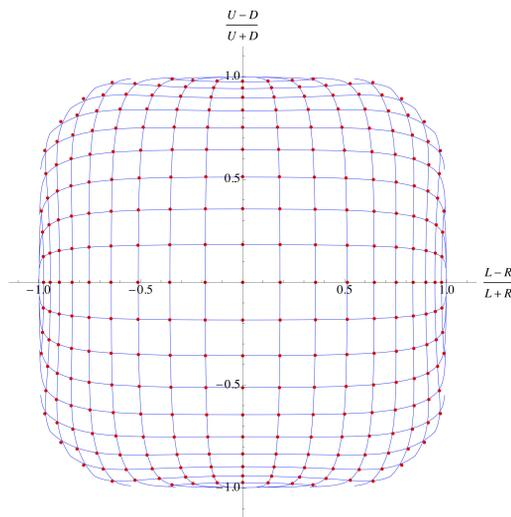
Figure 4: BPM response to the beam or wire. Blue lines are calculated response to the beam on the grid lines in Fig. 3. Dots are the results of the stretched-wire method measured with 10-mm step.
