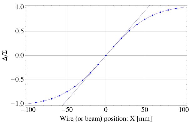
Figure 6: BPM response on the x-axis. Blue curved line: the calculated  $\Delta/\Sigma$  vs. the beam position, blue dots: the measured  $\Delta/\Sigma$  vs. the wire position, and blue straight line: a linear approximation at the origin.
